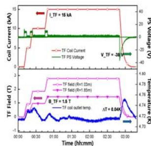
Fig. 7 Operating features of TF magnet
