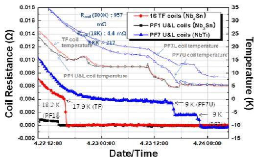
Fig. 6 SC transition of the KSTAR magnets
