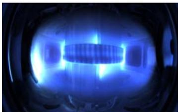
Fig.9 Image of ohmic discharge plasma
