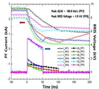
Fig. 8 Blip test results of PF magnets
