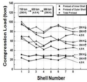
Fig.4 Cool-down history Fig.5 Pre-load change of CS
