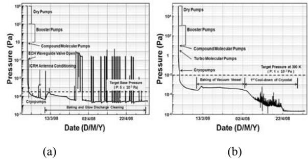
Fig. 3 Vacuum history (a) VV, (b) cryostat
