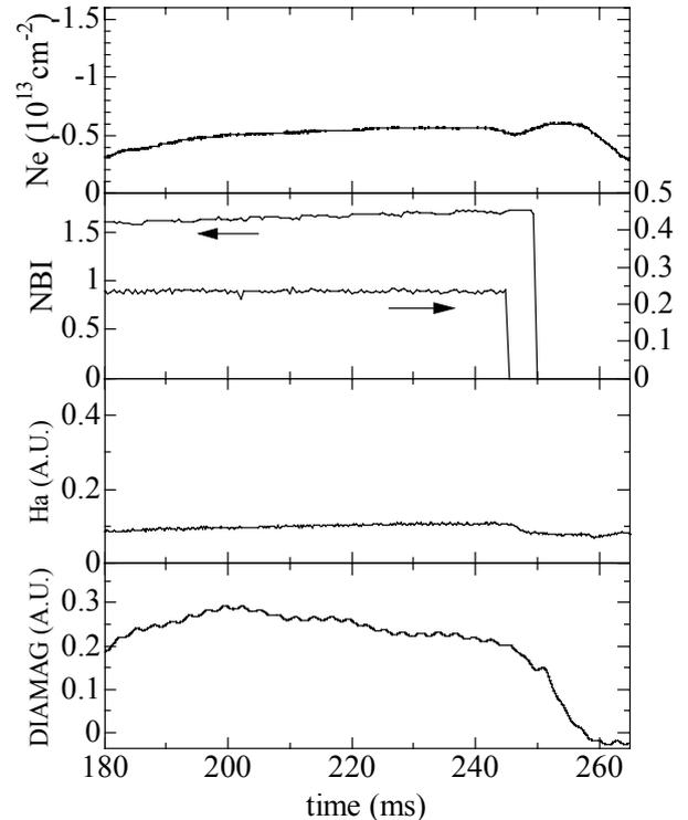
Fig.3 Typical waveform of Heliotron J plasma without SMBI (#32783)
