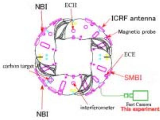
Fig.1 Top view of Heliotron J
