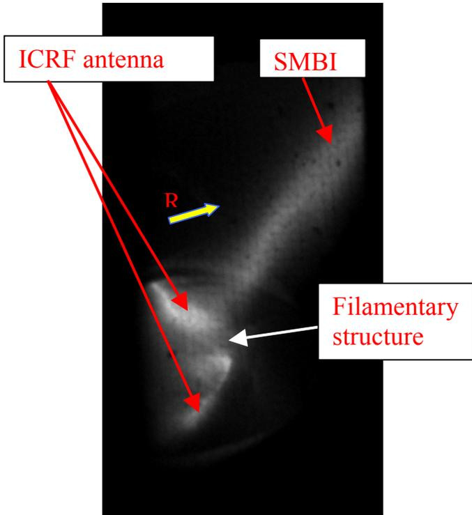
Fig.4 Fast camera image during SMBI
