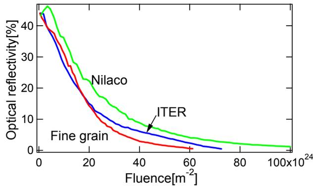
Fig. 5 Measured reflectivity of three samples which were manufactured by different procedure
