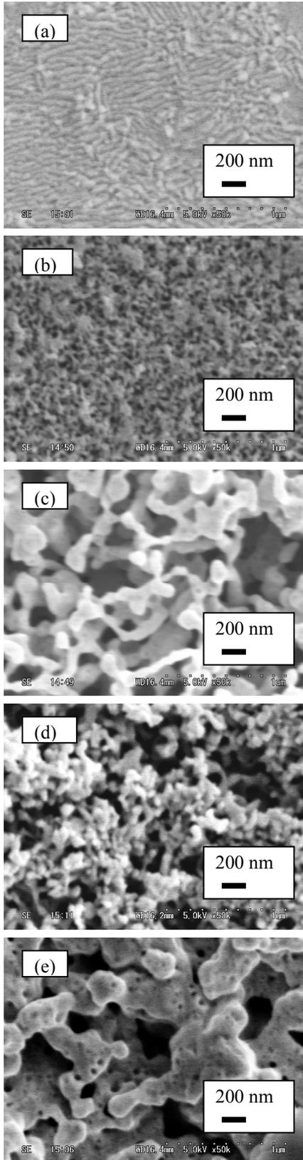
Fig. 3 SEM micrographs of the tungsten surface after the helium plasma exposure. The sample temperatures are (a) 900 K, (b) 1130 K, (c) 1400 K, (d) 1750 K and (e) 2040 K, respectively.
