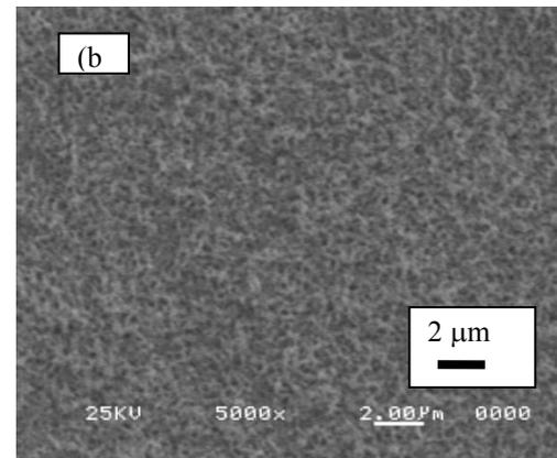
Fig. 6 SEM micrographs of tungsten surface (a) UFG and (b) ITER after helium plasma exposure.
