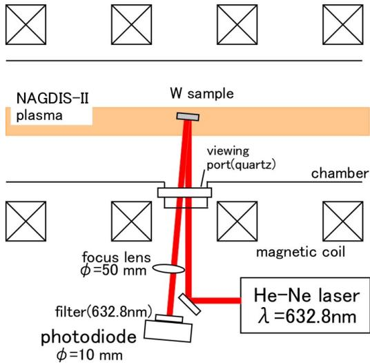
Fig. 1 Schematic illustration of the experimental setup in the divertor simulator NAGDIS-II.
