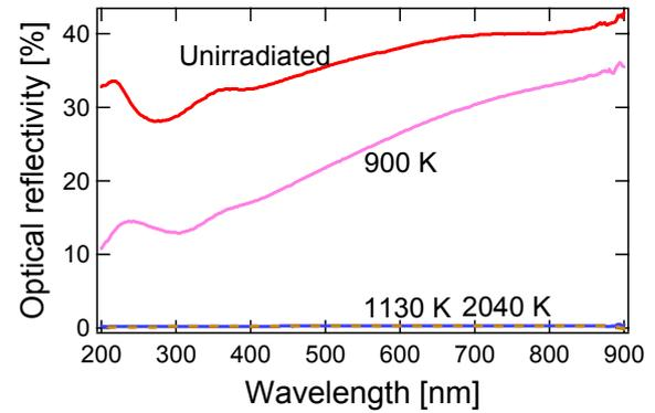
Fig. 4 Reflectivity of polished samples and samples irradiated at 900 K, 1130 K, 2040 K.
