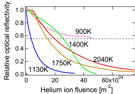
Fig. 2 Measured reflectivity of tungsten under helium plasma exposure at different sample temperatures from 900 K to 2040 K
