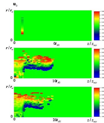
Fig.3 Color contours of azimuthal flow of the beam ions. (Top)  $t = 0$ , (middle)  $t = 10t_{A0}$ , and (bottom)  $t = 20t_{A0}$ .
