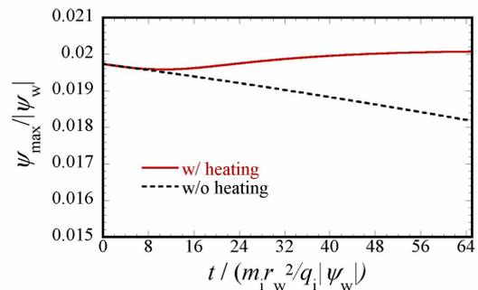
Fig.7 Time evolution of the maximum trapped flux. The red solid line shows flux supply by the electron heat generation. The flux decays resistively for the case of the black solid line.
