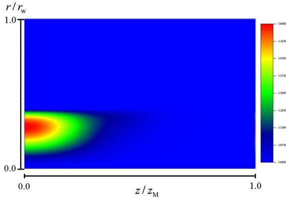
Fig.5 Color contour of the electron temperature at  $t = 18.7 t_{A0}$ . The maximum of the temperature reaches 1.6 times higher than the initial value.
