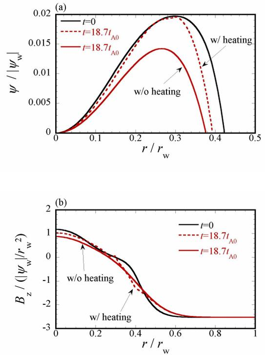
Fig.6 The midplane ( $z=0$ ) profiles of (a) the magnetic flux function and (b) the magnetic field. The black solid lines indicate the initial profiles.
