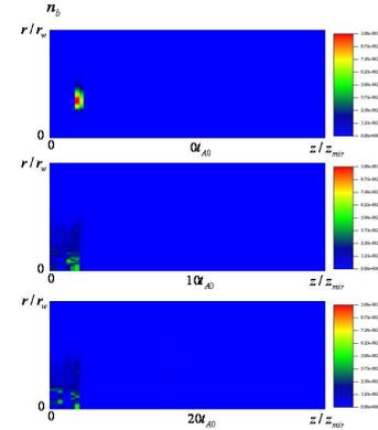
Fig.2 Color contours of the beam ion density. (Top)  $t = 0$ , (middle)  $t = 10t_{A0}$ , and (bottom)  $t = 20t_{A0}$ .
