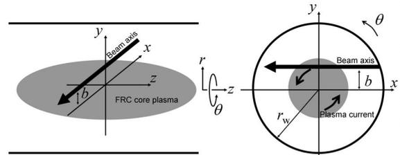
Fig.1 Geometry of tangential neutral beam injection.
