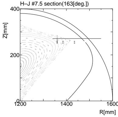
Fig. 1 Probe pins position of the Hybrid Directional Probe (HDP) on port 7.5 cross section. HDP head moves along horizontal solid line at  $Z = 0.271$ [m] with setting parameter  $R_p$ . Probe pins move along vertical dashed line at  $R = 1.36$ [m] with  $\alpha_p$ .
