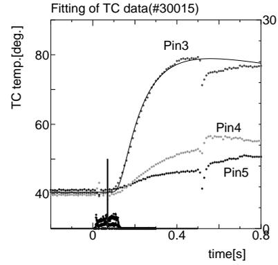
Fig. 2 Example of TC data and fitting result for the HDP. The position of Pins are  $R = 1.36$ [m](Pin3 and 4),  $1.38$ [m](Pin5), and  $Z = 0.25$ [m](Pin3 and 5),  $0.26$ [m](Pin4). Solid line fitting Pin3 data is obtained by eq.(1) with  $x_{tc} \sim 1.07 \times 10^{-2}$ [m] and  $q\Delta t \sim 2.9$ [J/mm<sup>2</sup>].
