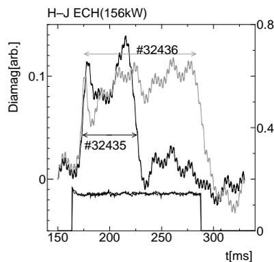
Fig. 5 Diamag monitor signal for two successive shot with the same ECH power and slightly different gas puffing control.
