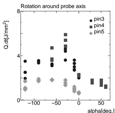
Fig. 3 Heat flux profile around HDP head. Horizontal axis is angle around HDP ( $\alpha$ ) and vertical axis is the heat received during whole discharge ( $q\Delta t$ ). For rotation angle  $\alpha_p = 0$ , Pin3 (and Pin5) is at  $\alpha = -10[\text{deg.}]$  and Pin 4 is at  $\alpha = 50[\text{deg.}]$ .
