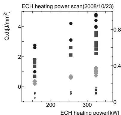
Fig. 4 ECH power scan effect on heat flux. Data symbols are the same as Fig. 3. Small open circles are also plotted for diamant monitor value (right axis with arbitrary unit).
