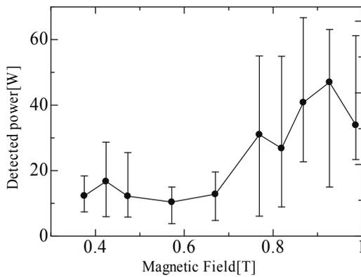
Fig.9 Output powers versus the magnetic field for a 50-period sinusoidal corrugated SWS. The beam voltage is about 40kV
