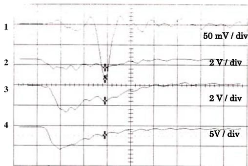
Fig.6 Waveform of measured signals: 1 microwave output, 2 cathode current, 3 beam current and 4 beam voltage.
