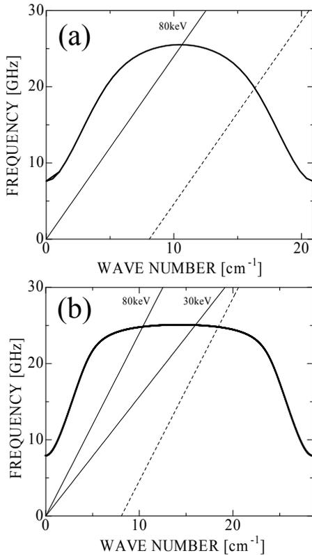
Fig.2 Dispersion characteristics of  $TM_{01}$  for rectangular SWS, (a) for A type SWS and (b) B type SWS. Solid lines and dashed lines are slow space charge mode and slow cyclotron mode, respectively.
