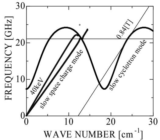
Fig.10 Dispersion curves of fundamental  $TM_{01}$  for type B SWS. The beam energy is 40 keV.
