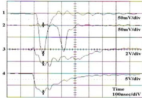
Fig.5 Waveform of measured signals: 1 prompt signal, 2 delayed signal, 3 beam current and 4 beam voltage.
