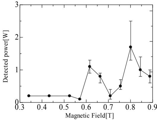
Fig.8 Output powers versus the magnetic field for a 10-period SWS of B type. The beam voltage is about 30kV.
