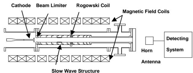
Fig.4 Schematic diagram of the experimental setup.
