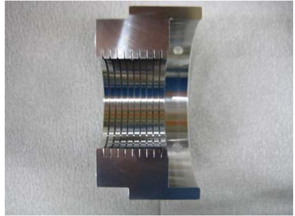
Fig.3 Rectangular corrugation of type B.
