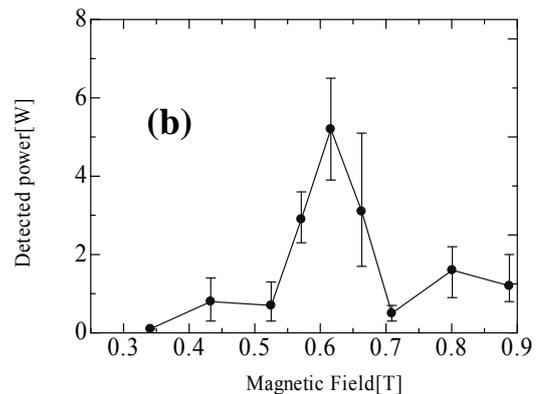
Fig.7 Output powers versus the magnetic field for a 10-period B SWS. The upper is the disk-integrated SWS and the lower is the improved SWS. The beam voltage is about 30kV.
