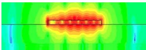
Figure 1. Excitation of plasmon in gold nanorod by the dipole source.
