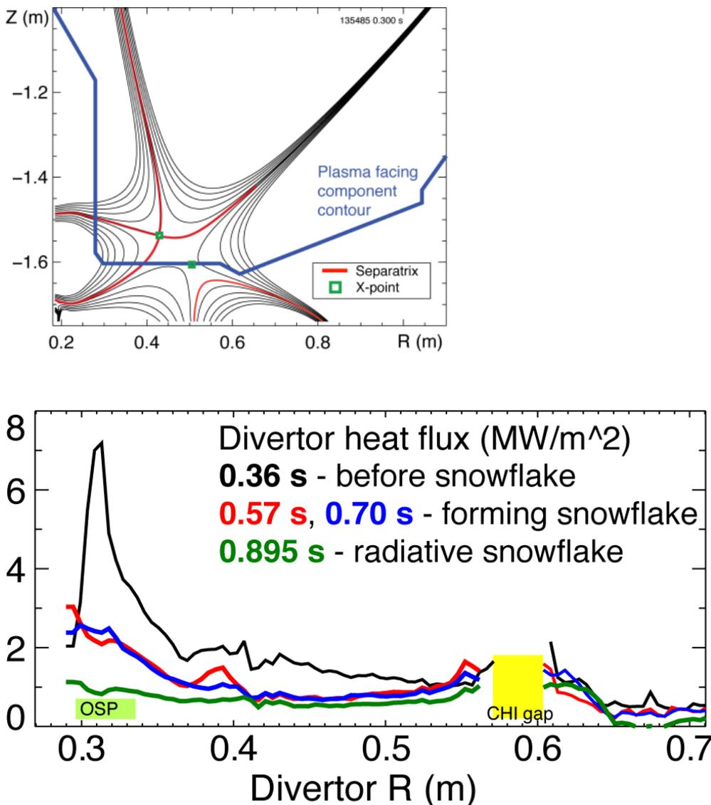
Figure 3: Top plot: Snowflake divertor configuration used in NSTX (M. Bell, I-1). Bottom plot: Measured heat flux before and during the snowflake configuration.
