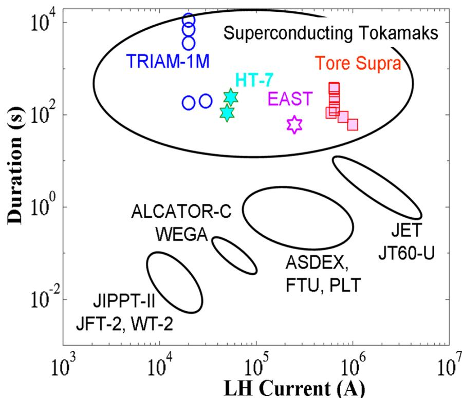
Figure 2: Overall results of long pulse operation of tokamaks with LHCD (T. Hoang I-6) (Reproduced from T. Hoang, Plasma and Fusion Research to be published)
