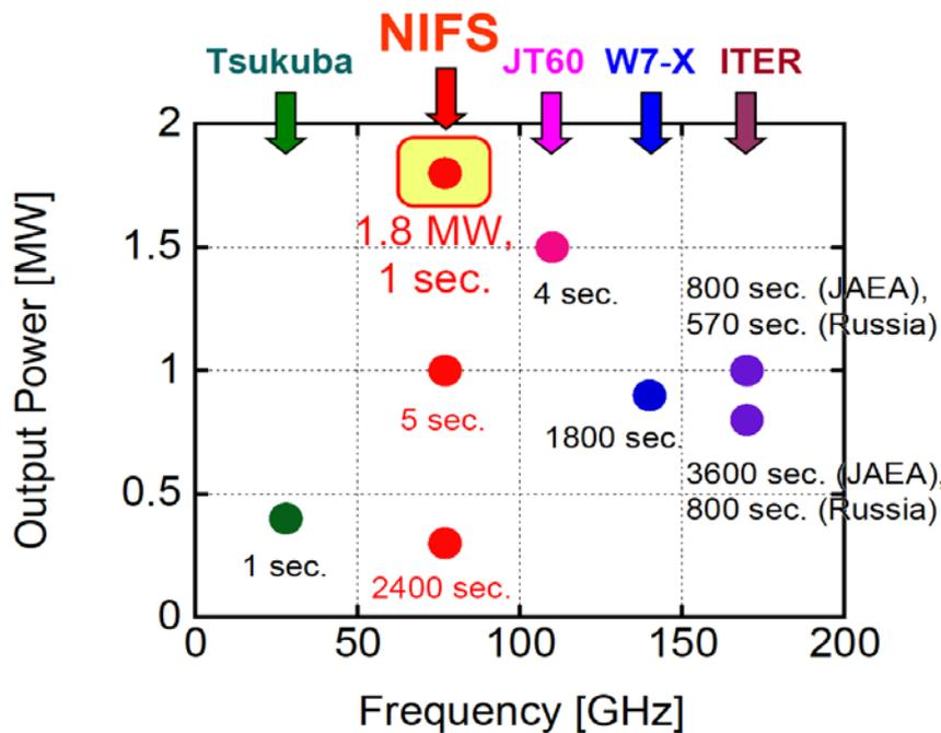
Figure 5: Status of long pulse operation of gyrotrons for magnetic fusion (T. Mutoh PL-1)
