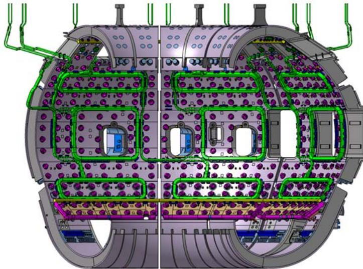
Figure 4: ITER internal coil design capable of producing a broad range of magnetic perturbations at the edge ( $n=1, 2, 3$  and  $4$ )
