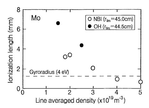
Fig.5 I onization length of Mo neutral determined by the decay length of MoI light intensity near the test limiter for OH plasma( ● ) and NBI plasma( ○ ). Gyroradius of Mo+ (4 eV) is about 1.3 mm.
