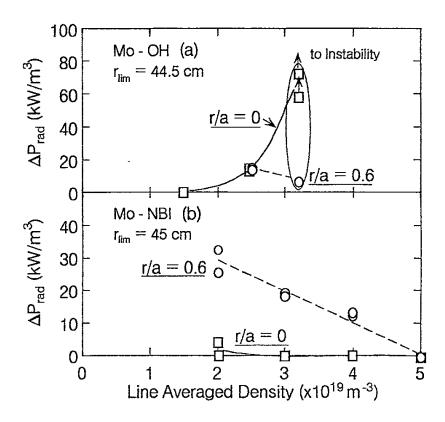
Fig. 2. Radiation increment  $\Delta P_{\rm rad}$  at the positions of the magnetic axis (r/a = 0, where a is the minor radius,  $\Box$ ) and at r/a = 0.6 ( $\bigcirc$ ) for OH plasma at  $r_{\rm lim}$  = 44.5 cm (a), and for NBI plasma at  $r_{\rm lim}$  = 45.0 cm (b).
