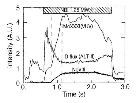
Fig. 3. Time evolution of D-flux from the ALT-II main limiter, a VUV line of MoXXXI (17.7 nm), and a NeVIII line for NBI plasma with  $\overline{n}_e$  of 3 x  $10^{19}$  m<sup>-3</sup> with neon cooling.
