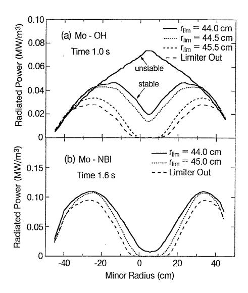
Fig. 1. Radial profiles of radiated power in OH(a) and in NBI(b) plasmas for different Mo limiter position ( $\overline{n}_e = 2.5 \times 10^{13} \text{ cm}^{-3}$ ).
