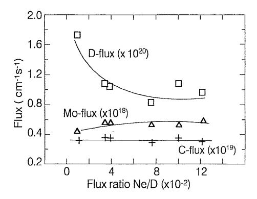
Fig. 4. D-, Mo- and C-fluxes on the Mo test limiter as a function of flux ratio of Ne/D. The fluxes are integrated in the poloidal direction (unit cm<sup>-1</sup>s<sup>-1</sup>).
