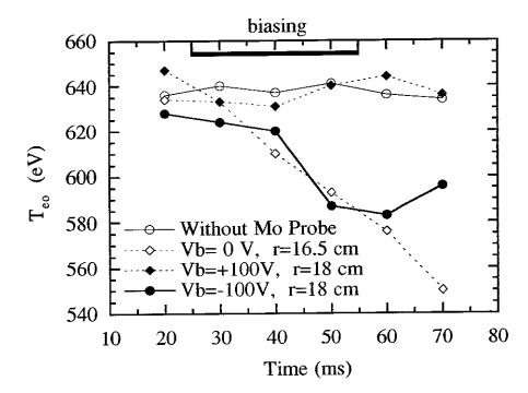
Fig. 3 Temporal behavior of the central electron temperature  $T_{e0}$  with the Mo probe inserted to 1.5 cm inside the LCFS, biased to  $\pm$  100 V. The signals at the same location without biasing and those without the Mo probe insertion are plotted as the reference.
