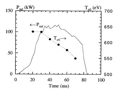
Fig. 2 Temporal behavior of the radiation loss  $P_{rad}$  and the central electron temperature  $T_{e\theta}$  with the Mo probe inserted to 3 cm inside the LCFS.
