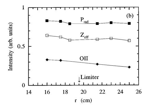
Fig. 1 Parameters measured as a function of the probe position  $\,r$ . Plasma current  $I_p$  was 66 kA, field strength  $B_T$  1.0 T,  $T_{e0}$  600 - 700 eV, average density  $n_e$  1.9 - 2.1 x  $10^{19}$ /m<sup>3</sup>.
