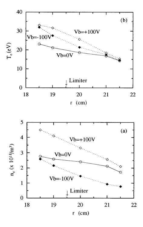
Fig. 4 Edge density (a) and temperature (b) profiles for positive and negative iasing. The bias voltage Vb was applied from 25 ms to 55 ms.
