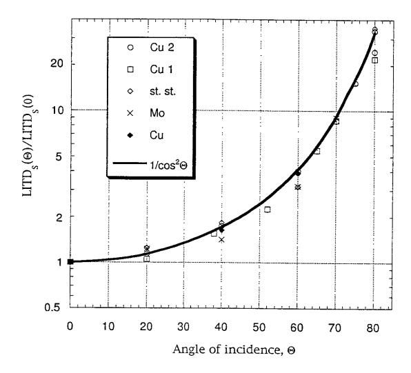
Fig. 5. Change of LIDT for s-polarised laser beam versus angle of incidence, after [22] and [31].
