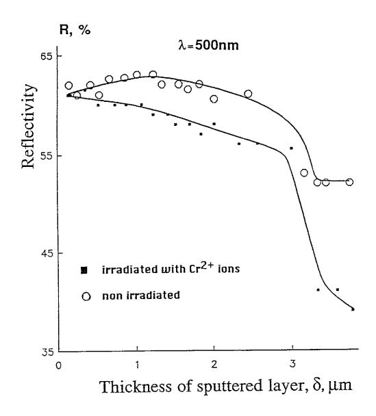
Fig. 6. (a) Dependence of reflectivity of stainless steel on the thickness of layer sputtered by ions of deuterium plasma.
