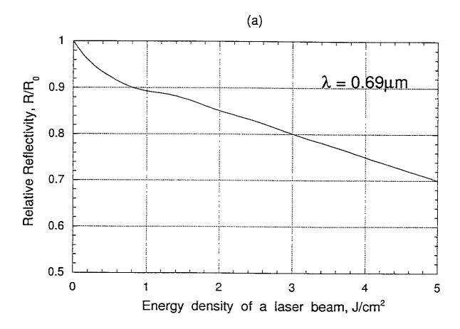
Fig. 3. (a) Dependence of reflectivity of copper mirrors during the laser pulse on the energy of laser beam for  $\lambda$ =0.69  $\mu$ m [26].
