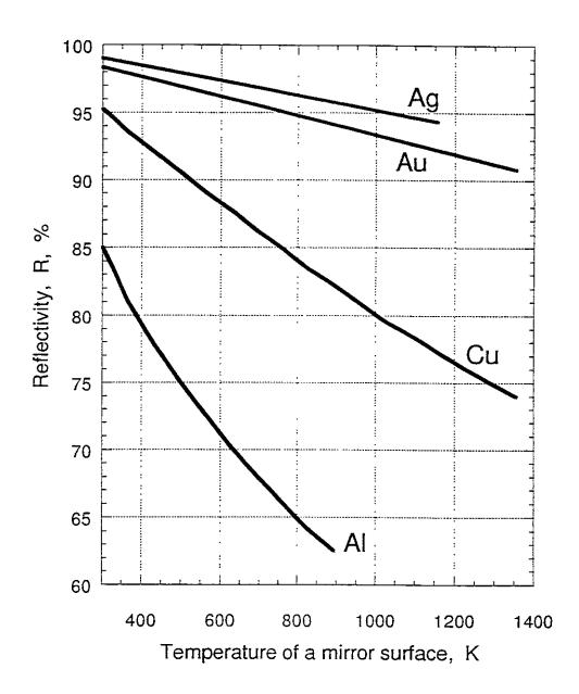
Fig. 1. Reflectivity of several metals at  $\lambda$ =1.064  $\mu$ m versus temperature of mirror surface [15].
