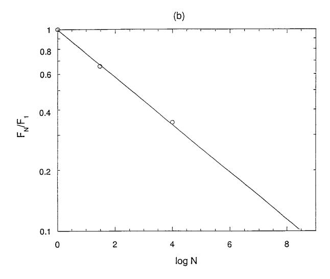
Fig. 4. (b) Change of LIDT values with increasing number of laser shots Mo [8].
