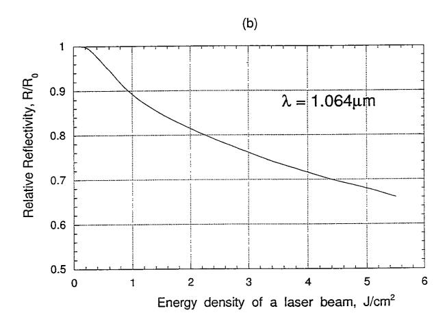
Fig. 3. (b) Dependence of reflectivity of copper mirrors during the laser pulse on the energy of laser beam for  $\lambda=1.064~\mu m$  [27].
