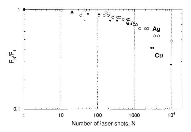
Fig. 4. (a) Change of LIDT values with increasing number of laser shots for Cu and Ag [23]. and (b) Mo [8].
