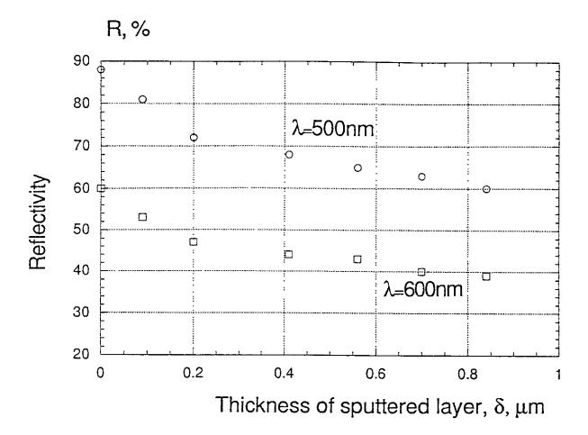
Fig. 6. (b) Dependence of reflectivity of copper mirrors on the thickness of layer sputtered by ions of deuterium plasma.
