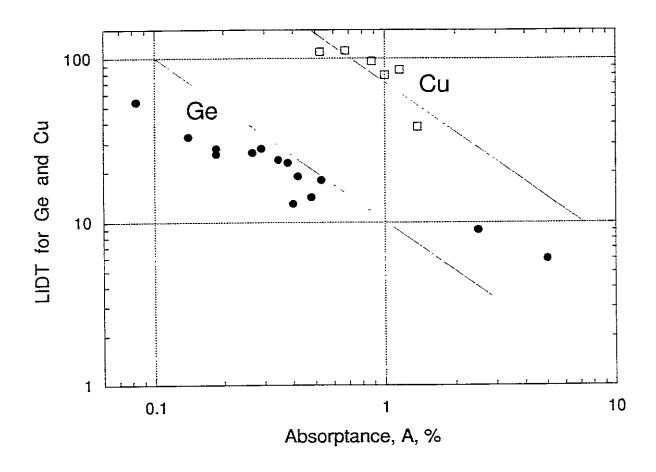
Fig. 2. Dependence of LIDT on the surface absorptivity of Ge at  $\lambda$ =10.6  $\mu$ m [25] and Cu at  $\lambda$ =1.064  $\mu$ m [10]. Lines show the A<sup>-1</sup> dependencies.
