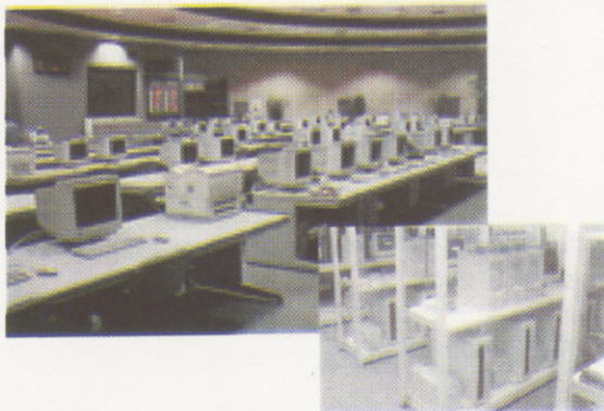
Figure 8: Photographs of Diagnostic client PCs in the Central Control Room (upper) and a cluster of server computers in the Diagnostics Computer Room (lower right)
