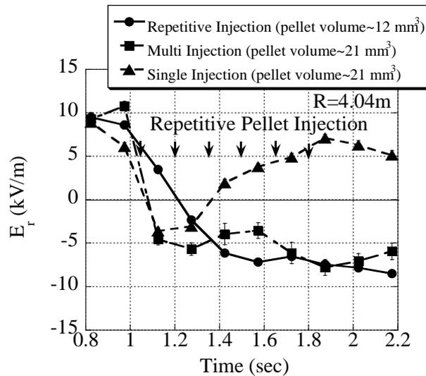
FIG.3. Time evolution of the radial electric field at the  $R=4.04$  with repetitive (circle), multi (square) and single pellet injection (triangle).
