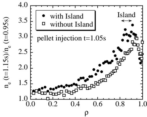
FIG.6. The radial profile of the ratio of electron density 0.1 sec after the pellet injection to that 0.1 sec before the pellet injection ( $t=1.05$ sec) in the plasma with and without the magnetic Island.
