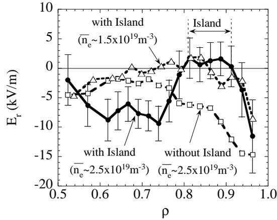
FIG.5. Radial profiles of  $E_r$  after the pellet injection in the plasmas with (closed circles) and without (open squares) magnetic island at high density and with magnetic island (open triangles) at low density.
