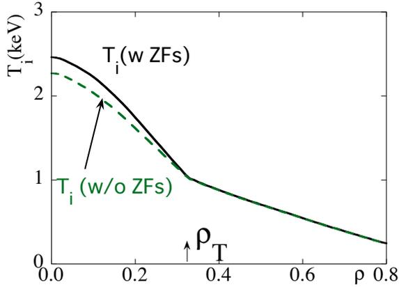
**FIG. 3.** Profiles of the ion temperature. The case with the effect of zonal flows is obtained (the solid line) and the case without the effect of zonal flows is shown (the dashed line), respectively.
