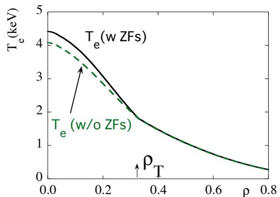
**FIG. 2.** Profiles of the electron temperature. Cases with the effect of zonal flows (the solid line) and without the effect of zonal flows are shown (the dashed line), respectively. The transport barrier can be obtained.
