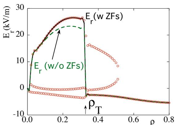
**FIG. 1.** Stationary profiles of the radial electric field as the result of the transport code. The solid line shows the case with the effect of zonal flows and the dashed line indicates the case without the effect of zonal flows.
