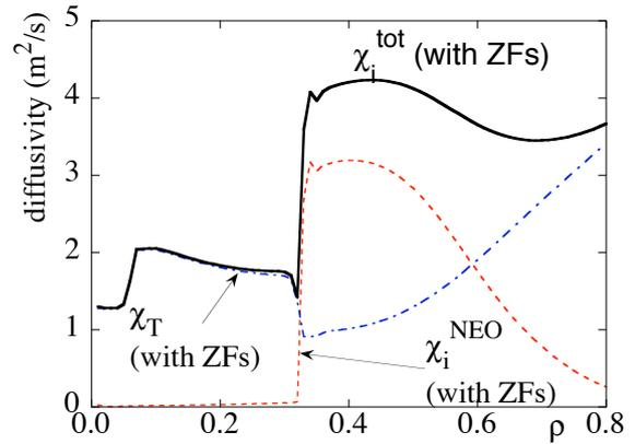
**FIG. 8.** Profile for the neoclassical heat diffusivity of ions with dashed line. The reduction of the neoclassical transport of ions is obtained in the region  $\rho < \rho_T$  due to the strong positive  $E_r$ .
