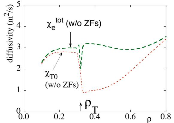
**FIG. 6.** Profiles of the heat diffusivity without the effect of the zonal flow
