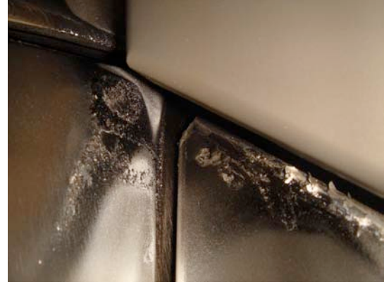
Fig.6 Thin metallic flakes on the graphite divertor plates.
