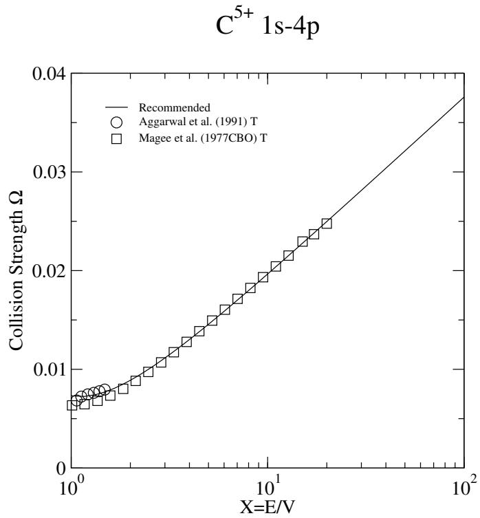
FIG. 13: Collision strength for electron-impact excitation.
