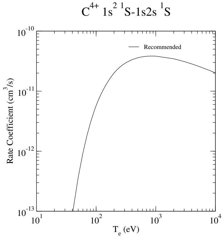
FIG. 20: Rate coefficient for electron-impact excitation.
