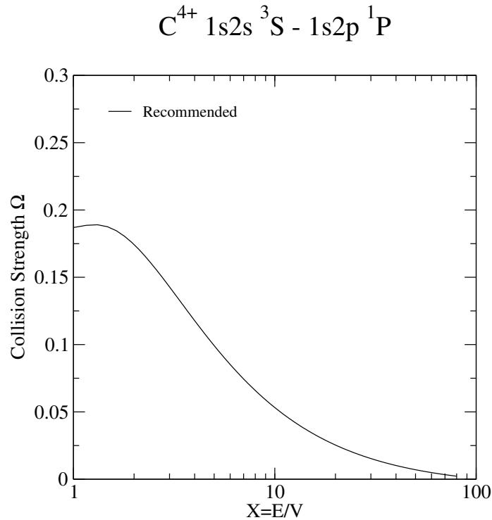
FIG. 33: Collision strength for electron-impact excitation.
