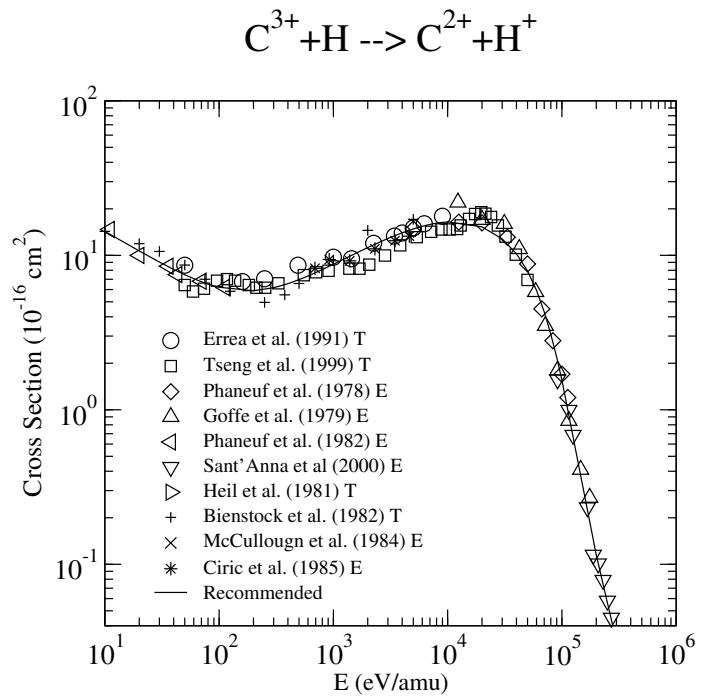
FIG. 172: Cross section for charge exchange.
