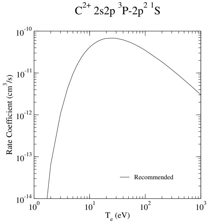
FIG. 80: Rate coefficient for electron-impact excitation.
