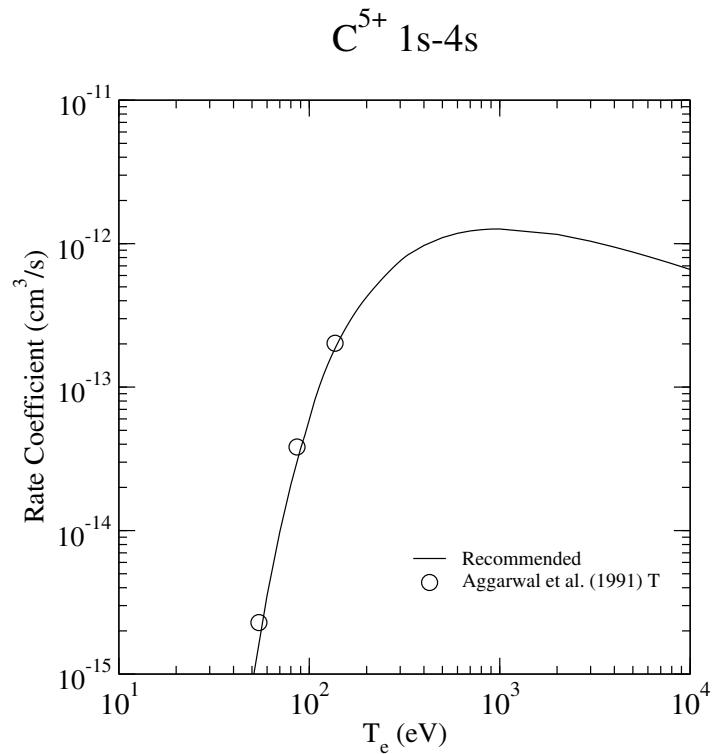
FIG. 12: Rate coefficient for electron-impact excitation.
