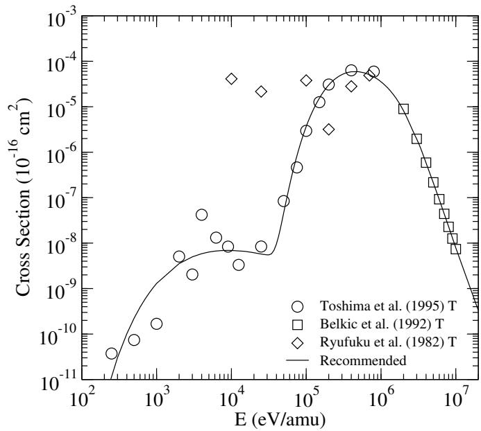
FIG. 139: Cross section for charge exchange.
