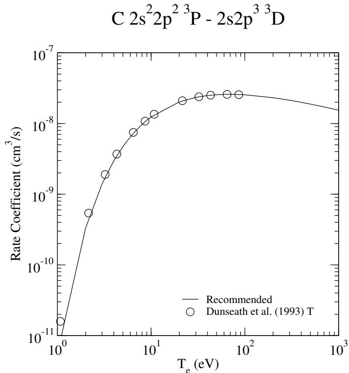
FIG. 118: Rate coefficient for electron-impact excitation.
