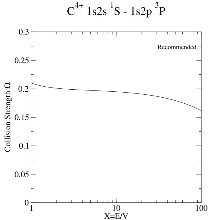
FIG. 37: Collision strength for electron-impact excitation.
