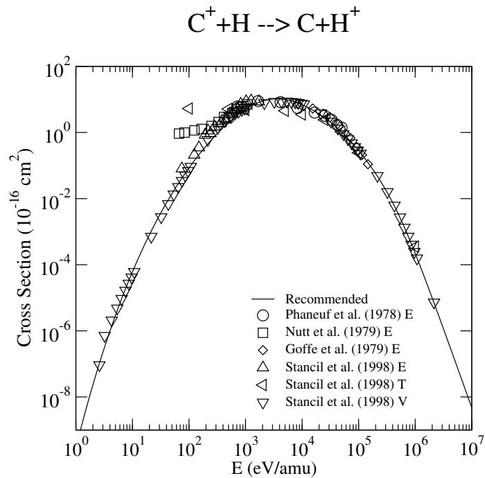
FIG. 174: Cross section for charge exchange.
