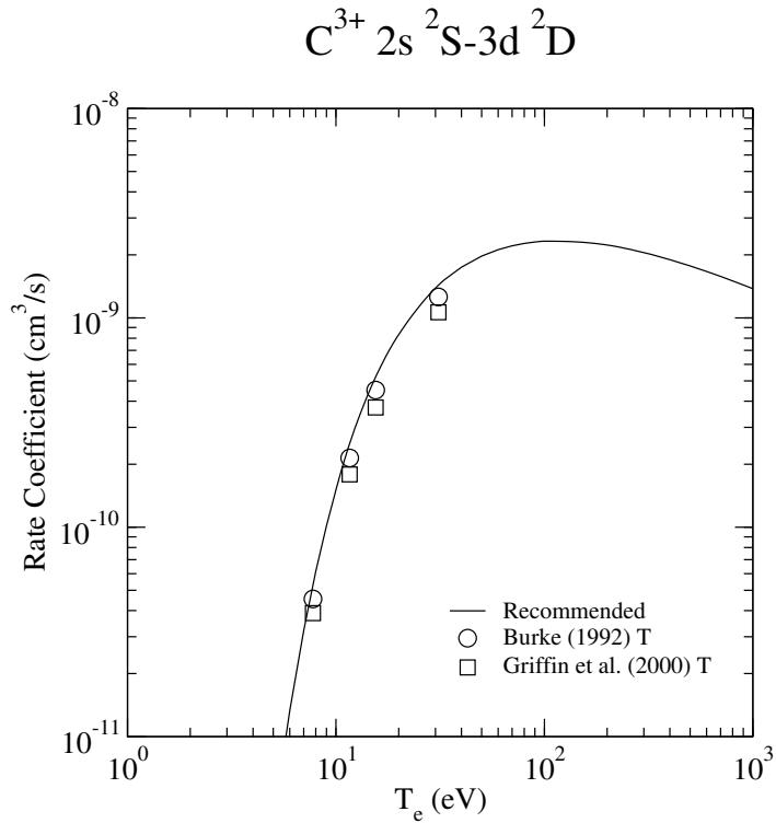
FIG. 52: Rate coefficient for electron-impact excitation.
