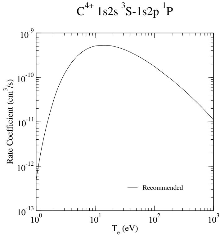
FIG. 34: Rate coefficient for electron-impact excitation.
