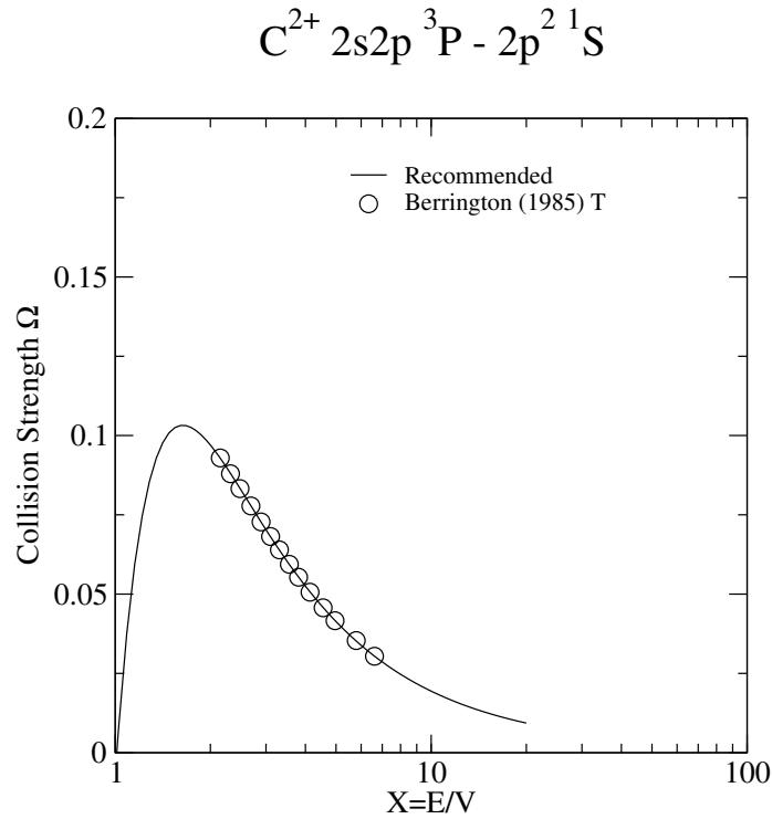
FIG. 79: Collision strength for electron-impact excitation.
