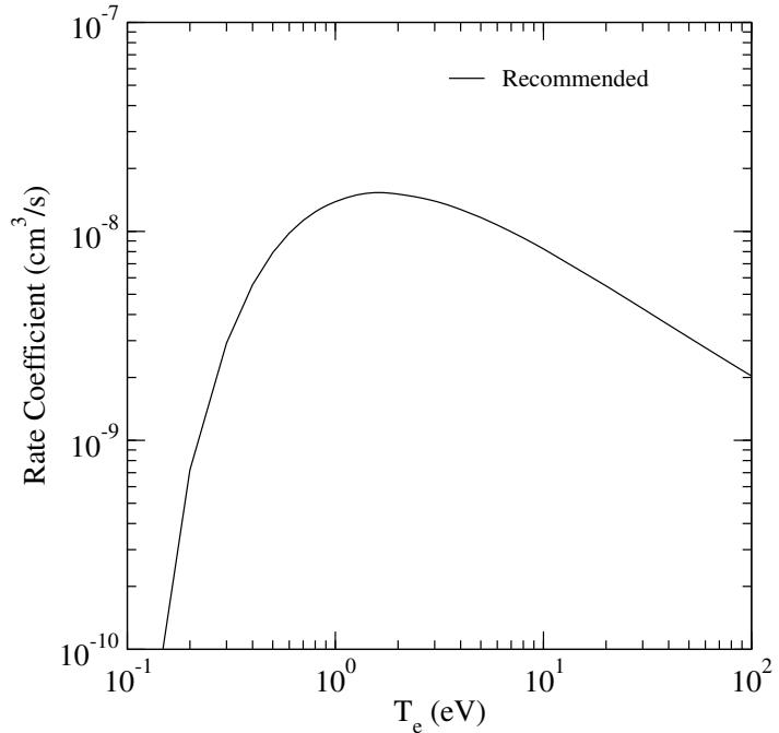
FIG. 78: Rate coefficient for electron-impact excitation.
