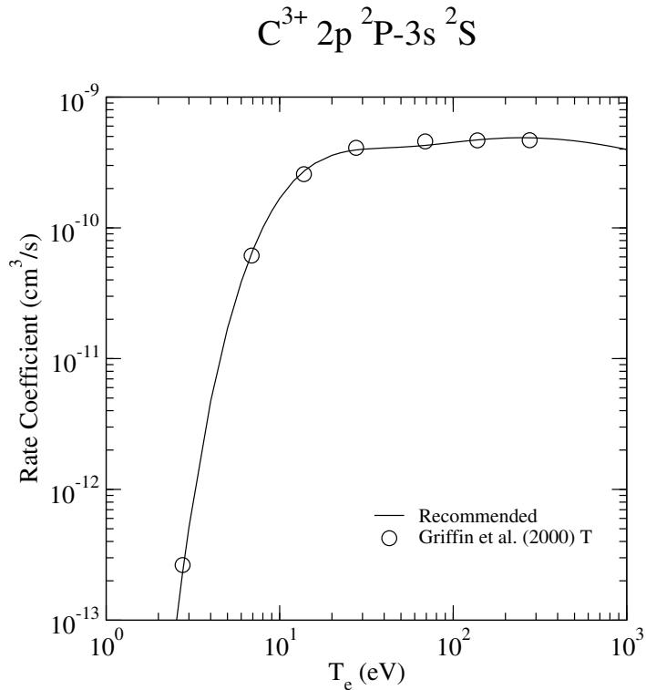
FIG. 56: Rate coefficient for electron-impact excitation.
