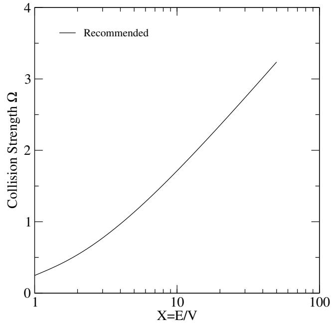
FIG. 35: Collision strength for electron-impact excitation.
