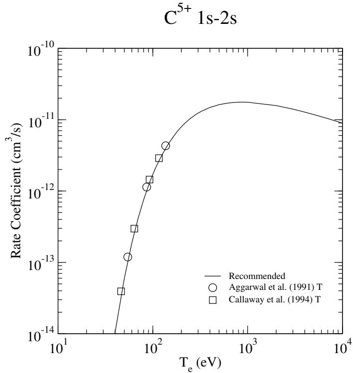
FIG. 2: Rate coefficient for electron-impact excitation.
