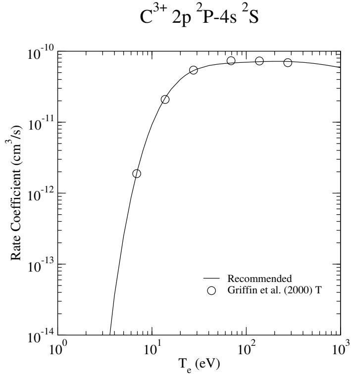
FIG. 60: Rate coefficient for electron-impact excitation.
