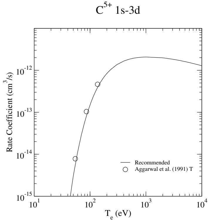
FIG. 10: Rate coefficient for electron-impact excitation.
