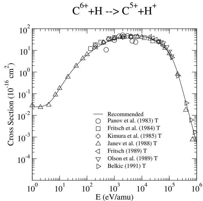
FIG. 158: Cross section for charge exchange.
