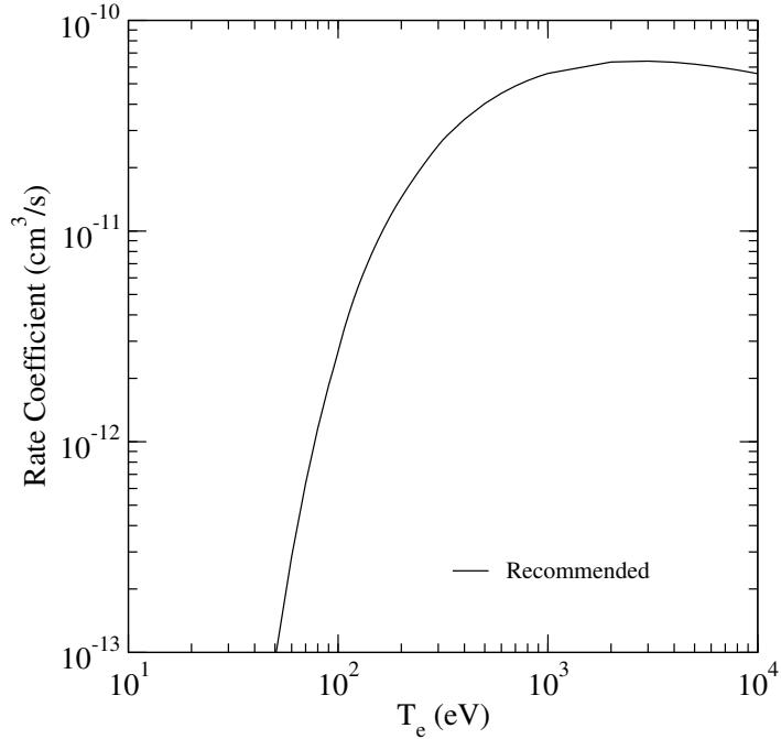
FIG. 28: Rate coefficient for electron-impact excitation.
