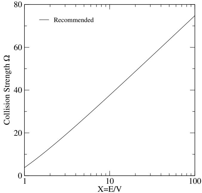
FIG. 99: Collision strength for electron-impact excitation.
