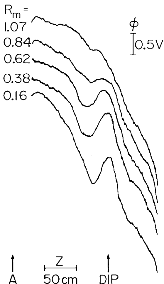
Fig.3. Potential profiles for magnetic dips. B_0 = 3.71 kG, P_{Ar} = 6.7 \times 10^{-3} Pa. Dip bottom is shown by arrow.
