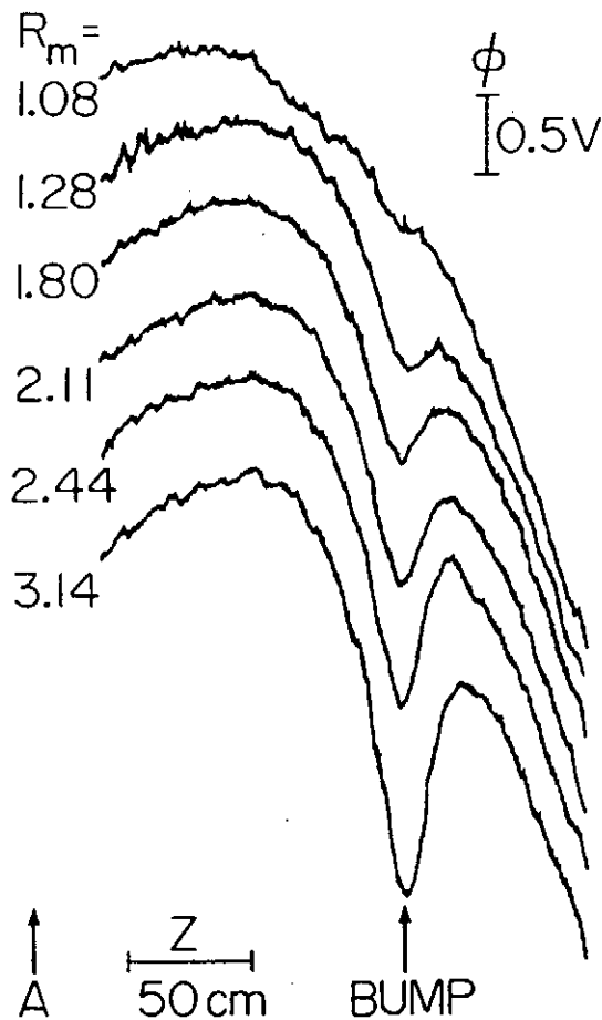
Fig.1. Axial potential profiles for magnetic bumps. B_0=1.24 \text{ kG} ; P_{\text{Ar}}=4.5 \times 10^{-3} \text{ Pa} . A is anode and the other arrow indicates bump top.
