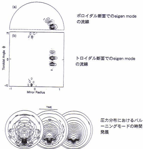
FIG. 4. The nonlinear time development of the pressure.
