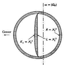
Fig.12.4 L cutoff layer  $(L = N_{\parallel}^2)$ , R cutoff layer  $(R = N_{\parallel}^2)$ , and the ion-ion hybrid resonance layer  $(K_{\perp} = N_{\parallel}^2)$  of ICRF wave in a tokamak with two ion components D<sup>+</sup>, H<sup>+</sup>. The shaded area is the region of  $N_{\perp}^2 < 0$ .
