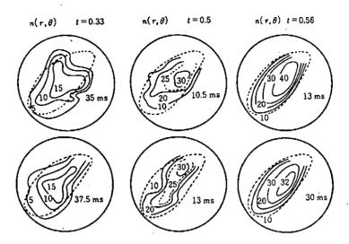
Fig.17.10 Equidensity contours of plasmas confined in JIPP I-b stellarator (l=2) with the rotational transform angles of  $\iota/2\pi=1/2,1/3$  and 0.56.<sup>38</sup>
