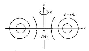
**Fig.6.1** Magnetic surfaces  $\psi = rA_{\varphi}$  and  $I(\psi)$
