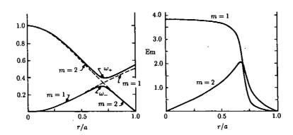
Fig.14.3 Lefthand-side figure: The toroidal shear Alfvén resonance frequencies  $\Omega$  that corresponds to (n=1, m=1) and (n=1, m=2),  $q(r) = 1 + (r/a)^2$ , a/R = 0.25,  $\Omega \equiv \omega/(v_A(0)/R_0)$ . Righthand-side figure: The structure of the global mode amplitude as a function of radius.
