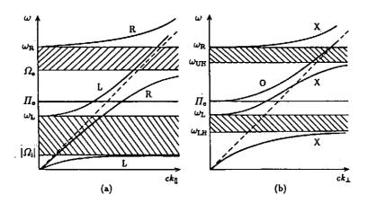
Fig.10.3 (a) Dispersion relations  $(\omega - ck_{\parallel})$  for R and L waves propagating parallel to the magnetic field  $(\theta = 0)$ , (b) Dispersion relations  $(\omega - ck_{\parallel})$  for O and X waves propagating perpendicular to the magnetic field  $(\theta = \pi/2)$ .
