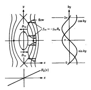
Fig.16.21 Tearing mode structure in the singular layer
