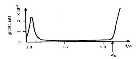
**Fig.16.28** The growth rate  $\gamma_{\rm res}(d)$  versus resistive wall position d/a in the case of  $\omega_{\rm rot} = 0.5$ .  $\gamma_{\rm res}(d)$  and  $\omega_{\rm rot}$  are in unit of  $\tau_{\rm A}^{-1} = B/(a(\mu_0\rho)^{1/2}) = (B/B_\theta)\tau_{\rm A\theta}^{-1}$ ,  $d_{\rm cr} = 2.115$ .  $(R/a = 5, q_0 = 1.05, m=2, n=1, \tau_{\rm A}/\tau_{\rm w} = 5 \times 10^{-4})$ . (Afer ref.50).
