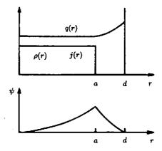
**Fig.16.25** Upper figure: Profiles of mass density  $\rho(r)$ , current density j(r) and q profile q(r). The plasma radius is r = a and the wall is located at r = d. Lower figure: Profile of flux function  $\psi(r)$  in the case of conducting wall.
