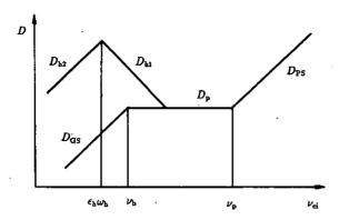
Fig.17.9 Dependence of the neoclassical diffusion coefficient of helical field on collision frequency.  $\nu_{\rm p} = (\iota/2\pi)v_{\rm Te}/R, \ \nu_{\rm b} = \epsilon_{\rm t}^{3/2}\nu_{\rm p}, \ \omega_{\rm h} = \epsilon_{\rm h}\kappa T_{\rm e}/(qBr^2).$
