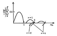
Fig.8.9 The relation of the growth rate  $\gamma$  and  $nq_a$  for kink instability  $(-2W/(\pi\xi_a^2B_a^2/\mu_0) = \gamma^2a^2(\langle\rho_{m0}\rangle\mu_0/B_a^2))$ . After V. D. Shafranov: Sov. Phys. Tech. Phys. 15, 175 (1970).
