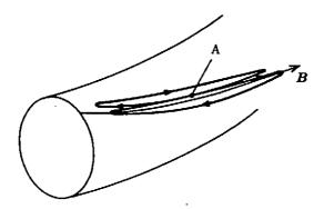
Fig.16.20 Banana orbits of trapped electrons those induce the bootstrap current
