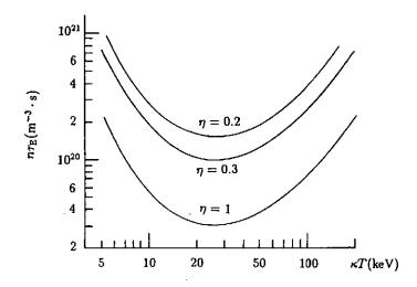
Fig.1.4 Condition of D-T fusion core plasma in  $n\tau_{\rm E}$ -T diagram in the case of  $\eta = 0.3$ , critical condition  $(\eta = 1)$  and ignition condition  $(\eta = 0.2)$ .
