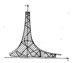
Fig.3.4 The dotted lines are lines of magnetic force and the solid lines are particle orbit in cusp field.
