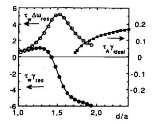
Fig.16.29 The growth rate  $\gamma_{\rm res}$  and slip frequency  $\Delta\omega_{\rm slip} = \omega_{\rm rot} - \omega_{\rm res}$  of resistive wall mode and the growth rate  $\gamma_{\rm ideal}$  of plasma mode versus resistive wall radius d/a for n=1.  $\omega_{\rm rot} = 0.06$  is unit of  $\tau_{\rm A}^{-1} = B/(a(\mu_0\rho)^{1/2}) = (B/B_\theta)\tau_{\rm A}^{-1}$ . (Afer ref.51).
