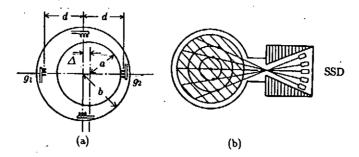
Fig.16.4 (a) Locations of magnetic probes around plasma ( $\Delta$  shown in the figure is minus) (b) an array of soft X ray solid-state detectors. Each detector's main contribution to a signal comes from the emission at the peak temperature along the line of sight of the detector. the fluctuation of the electron temperature at this point can be detected.
