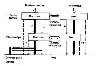
**Fig.16.13** Energy flow of ions and electrons in a plasma. Bold arrows, thermal conduction  $(\chi)$ . Light arrows, convective loss (D). Dashed arrow, radiation loss (R). Dot-dashed arrows, charge exchange loss (CX).
