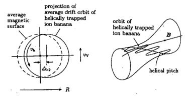
Fig.17.8 Orbit of helical banana ion trapped in helical ripple.
