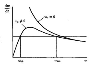
Fig.16.24 The curve of (16.81').  $w_{\rm th}$  is the threshold width of island for the onset of neoclassical tearing mode and  $w_{\rm sat}$  is the saturated width.
