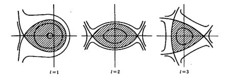
Fig.17.3 Magnetic surfaces, showing separatrix points and separatrices, of the helical field.
