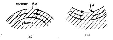
Fig. 8.2 Centrifugal force due to the curvature of magnetic-force lines.
