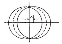
Fig.7.2 Magnetic surface (dotted line) and drift surfaces (solid lines).
