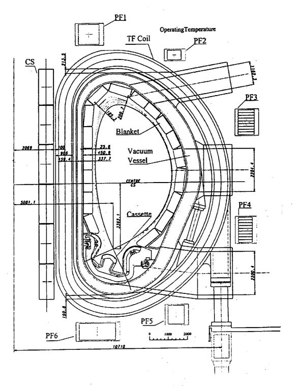
Fig.16.32 Toroidal cross section of ITER-FEAT outline design in 2000.
