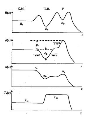
Fig.17.16 The magnitudes of magnetic field B(z), electrostatic potential  $\phi(z)$ , density n(z), and electron temperature  $T_{\rm e}(z)$  at the thermal barrier. C.M., central mirror. T.B., thermal barrier. P, plug mirror.
