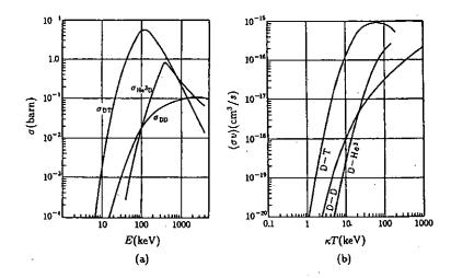
Fig.1.2 (a) The dependence of fusion cross section  $\sigma$  on the kinetic energy E of colliding nucleous.  $\sigma_{\rm DD}$  is the sum of the cross sections of D-D reactions (1) (2). 1 barn=10<sup>-24</sup> cm<sup>2</sup>. (b) The dependence of fusion rate  $\langle \sigma v \rangle$  on the ion temperature  $T_{\rm i}$ .
