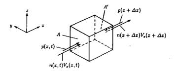
Fig.5.1 Particle flux and force due to pressure
