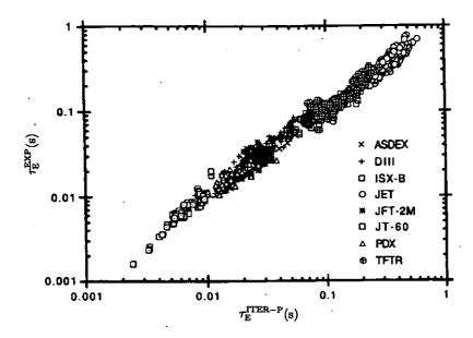
Fig.16.14 Comparison of confinement scaling  $\tau_{\rm E}^{\rm ITER-P}$  with experimental data of energy confinement time  $\tau_{\rm E}^{\rm EXP}$  of L mode. (After Yushimanov et al: Nucl. Fusion 30, 1999, (1990). ref.20)
