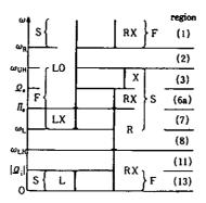
Fig.10.4 The  $\omega$  regions of R and L waves at  $\theta=0$ ; O and X waves at  $\theta=\pi/2$ ; F and S waves; in the case ( $\omega_{\rm L}<\Pi_{\rm e}<\Omega_{\rm e}$ ). The numbers on the right identify regions shown in the CMA diagram, fig.10.5.
