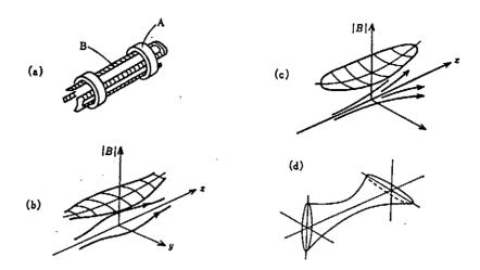
Fig.17.12 Minimum-B mirror field. (a) Coil system with mirror coil (A) and stabilizing coils (Ioffe bars) (B). (b) Magnitude of the magnetic field in a simple mirror. (c) Magnitude of the magnetic field in the minimum-B mirror field. (d) The shape of a quadrupole minimum-B (fishtail).
