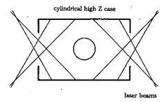
Fig.18.4 Structure of hohlraum target.
