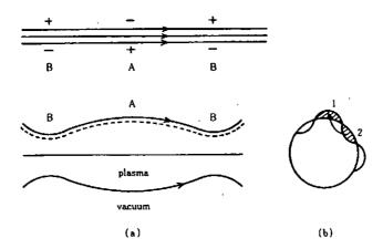
Fig.8.4 Charge separation in interchange instability. (a) The lower figure shows the unstable part A and the stable part B along a magnetic line of force. The upper figure shows the charge separation due to the acceleration along a flute. (b) Cross section of the perturbed plasma.
