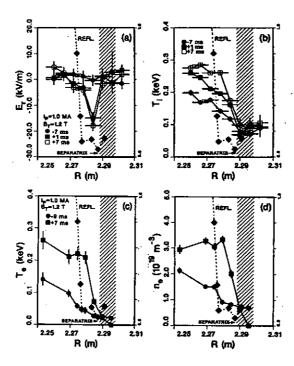
Fig.16.15 Plots of various edge plasma profiles at times spanning the L-H transition in DIHD. (a)  $E_r$  profile, (b) Profiles of the ion temperature measured by CVII charge exchange recombination spectroscopy, (c)(d) Profiles of electron temperature and electron density measured by Thomson scattering. (After Doyle et al: Plasma Phys. Controlled Nuc. Fusion Research 1, 235, (1991) IAEA. ref.24)
