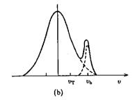
Fig.2.1 (a) Velocity space distribution function of Maxwellian with electron temperature  $T_{\rm e}$ . (b) velocity space distribution function of Maxwellian plasma with electron temterature  $T_{\rm e}$  and injected electron beam with the average velocity  $v_{\rm b}$ .
