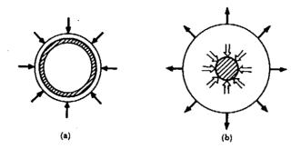
Fig.18.1 Conceptual drawing of implosion. (a) Irradiation by laser or particle beam from all side. (b) Expansion of plasma from the pellet surface and the implosion due to the reaction of the outward plasma jet.
