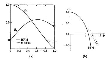
**Fig.17.1** (a) Toroidal field  $B_z(r)$  and poloidal field  $B_\theta(r)$  of RFP. The radial profiles of the Bessel function model (BFM) and the modified Bessel function model (MBFM) are shown. (b) F- $\Theta$  curve
