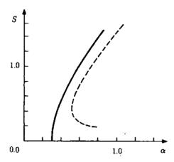
Fig.8.12 The maximum stable pressure gradient  $\alpha$  as a function of the shear parameter S of ballooning mode. The dotted line is the stability boundary obtained by imposing a more restricted boundary condition on the perturbation.<sup>16</sup>
