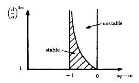
**Fig.16.26** Stable region in nq - m - d/a-diagram.
