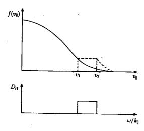
Fig.16.18 Distribution function  $f(v_{\parallel})$  of electrons is flatten in the region from  $v_1 = c/N_1$  to  $v_2 = c/N_2$  due to the interaction with the lower hybrid wave whose spectra of parallel index  $N_{\parallel}$  ranges from  $N_1$  to  $N_2$ .
