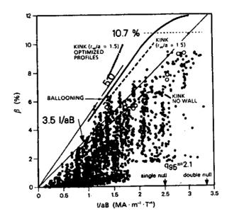
Fig.16.9 The observed beta versus I/aB for DIII-D. Various  $\beta$  limit calculations are summarized in the curves with different assumptions on the location of a conducting wall  $(r_w/a)$ . (After DIII-D team: Plasma Phys. Controlled Nuc. Fusion Research 1, 69, (1991) IAEA. ref.17)
