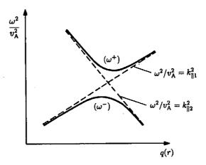
Fig.14.2 The dispersion relation of toroidally coupled m and m+1 modes.
