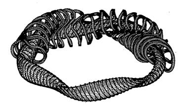
Fig.17.6 (a) Schematic view of the LHD device in Toki (R=3.9m,  $a \sim 0.6$ , B=3T). (b) Modular coil system and a magnetic surface of the optimized stellerator Wendelstein 7-X in Greifswald (R=5.5m, a=0.55m, B=3T).
