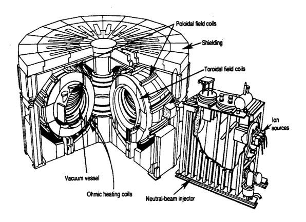
Fig.16.3 A birdview of TFTR( Tokamak Fusion Test Reactor), Plasma Physics Laboratory, Princeton University.
