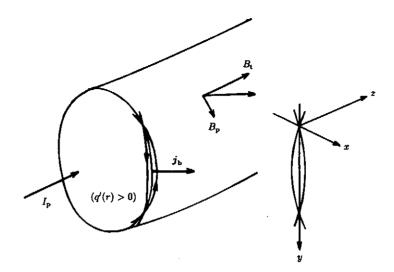
Fig.16.23 The coordinates in slab model and the coordinates in toroidal plasma. The coordinates (x,y,z) correspond radial coordinate  $r-r_{\rm s}$ , poloidal coordinate  $r\theta$  and toroidal coordinate  $R\varphi$  in toroidal plasma respectively. The arrows in the island indicate the direction of magnetic field  $B_{\rm p}-({\rm n}r/{\rm m}R)B_{\rm t}$  (refer eq.(16.79)).
