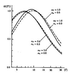
**Fig.16.30**  $\Theta$  is function of average temperature  $\langle T \rangle$  in cases with profile parameters  $(\alpha_T = 1.0, \alpha_n = 0.0), (\alpha_T = 2.0, \alpha_n = 0.0), (\alpha_T = 1.0, \alpha_n = 0.5)$  and  $(\alpha_T = 2.0, \alpha_n = 0.3)$
