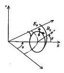
Fig.3.10 Coordinate system for explanation of Ware's pinch.
