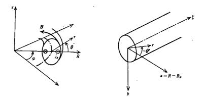
**Fig.6.9** Pfirsch-Schlüter current  $j_{\parallel}$  in a toroidal plasma.
