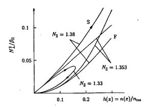
Fig.12.5 Trace of lower hybrid wave in  $N_\perp^2 - h(x) \, (= \Pi_{\rm e}^2(x)/\Pi_{\rm res}^2)$  diagram for the case of  $p=0.353,\ N_{\parallel c}^2=1+p=1.353$ . This corresponds to the case of H<sup>+</sup> plasma in  $B=3\,{\rm T},$  and  $f=\omega/2\pi=10^9\,{\rm Hz}.$  The electron density for the parameter  $\beta_\Pi=7.06\times 10^3\ (=\Pi_{\rm res}^2/\omega^2)$  is  $n_{\rm res}=0.31\times 10^{20}\,{\rm m}^{-3}.$
