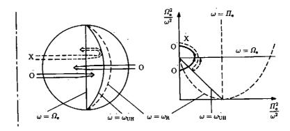
Fig.12.7 The locations of electron cyclotron resonance ( $\omega = \Omega_{\rm e}$ ), upperhybrid resonance ( $\omega = \omega_{\rm LH}$ ) and R cut off ( $\omega = \omega_{\rm R}$ ) in case of  $\Omega_{\rm e0} > \Pi_{\rm e0}$ , where  $\Omega_{\rm e0}$  and  $\Pi_{\rm e0}$  are electron cyclotron resonance frequency and plasma frequency at the plasma center respectively (left figure). The right figure is the CMA diagram near electron cyclotron frequency region.
