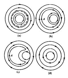
Fig. 16.8 The hot core in the center is expelled by the reconnection of magnetic surfaces
