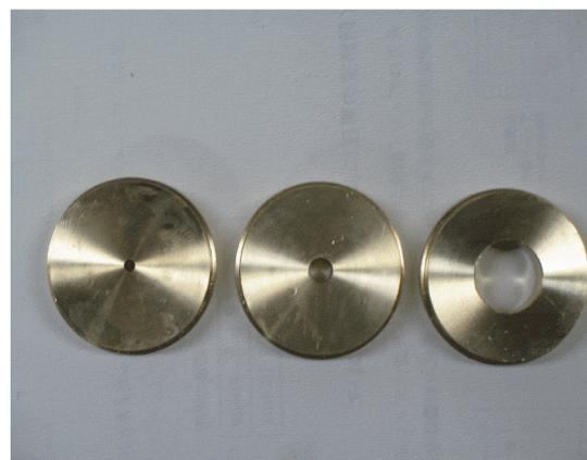
Fig.6. High pass filters.
