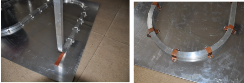
Figure 9: Details of the thermal shield pipe & plate connection
