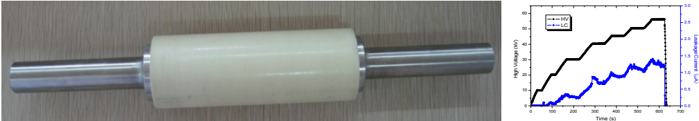
Figure 6: Insulator prototype and 56 kV HV test result
