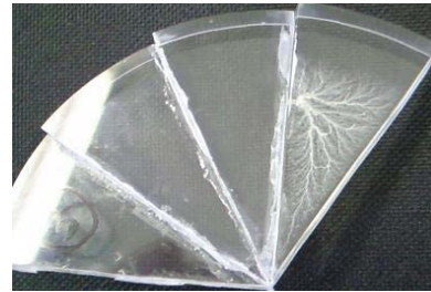
Fig. 5. Electron damage recorded on acrylic-resin plates.
