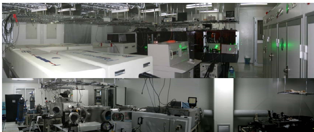
Figure 1: The Extreme Light III(XL-III) in Institute of Physics (IoP), Chinese Academy of Sciences, Beijing, China. This Ti:sapphire laser facility was designed with top-able configuration and can output peak power to 350TW with pulse duration of 30fs per 20 minutes. With further upgrade works by using OPCPA as front stage amplifier and optimized multipass amplifiers in recent, now the facility is able to delivery laser pulse to 750TW, contrast ratio about 10^{-8} , central wavelength at 810nm, focused laser intensity up to 10^{21} W/cm 2 . Upper: 527nm Nd:glass pump laser and 750TW Ti:sapphire facility. Bottom: Laser target chamber and diagnostic system (provided by Z.Y. Wei).
