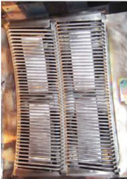
Fig.20 ICRF heating antenna with two straps
