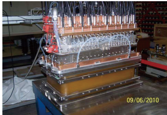
Fig.4 Ion source of NBI in ASIPP
