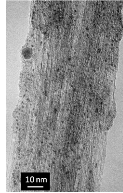
Fig. 11: TEM image of AuNPs synthesized using the CNTs as a template. P_{\text{gas}} = 60 \text{ Pa} , I_{\text{D}} = 1 \text{ mA} , t = 10 \text{ min} .
