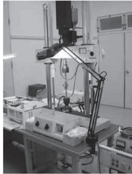
Fig. 1 Test apparatus for servo-controlled fatigue testing machine (maximum for fatigue; \pm 5 kN).
