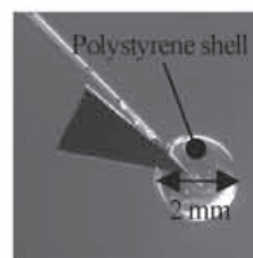
Fig. 2. Dummy target with a polystyrene shell.
