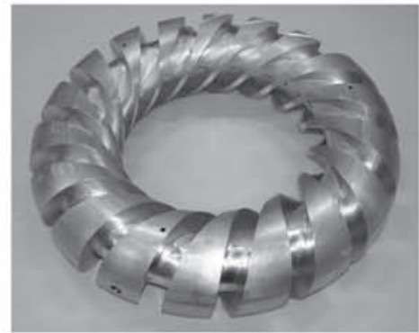
Figure 3: Winding form for the model coil.
