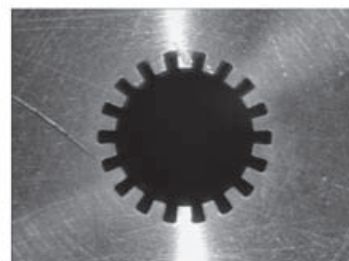
Fig.2 Structure of resonant cavity with 18-vane.
