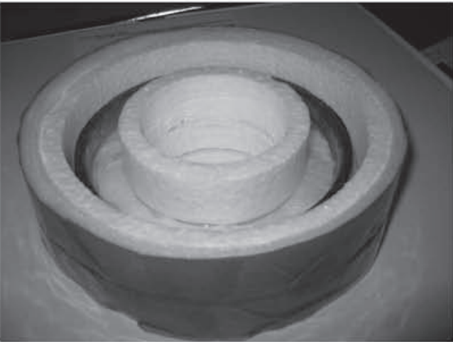
Fig. 1. A photo of FB-RT coil made of a YBCO tape.
