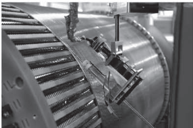
Fig. 25 The twist angle detector utilizing a reflective photo-interrupter
