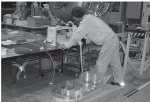
Fig. 17 Snap shot of the vacuum leak test in the Plasma Diagnostic Laboratories
