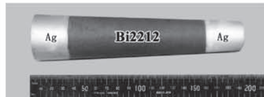
Fig. 1. Bi2212 HTS conical tubular conductor with Ag contact joint on both ends.
