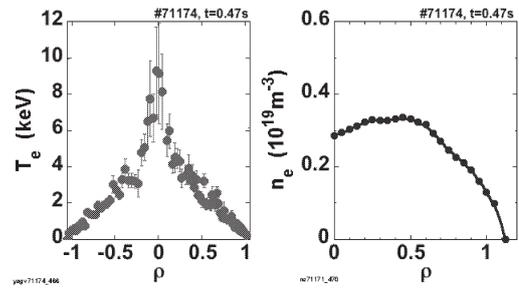
Fig. 1: Electron temperature and density profiles of high  $T_e$  shot.
