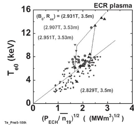
Fig. 2: Attained  $T_{e0}$  is plotted as a function of square root of ECH power normalized average density for different magnetic configurations. Small closed circles correspond to  $B_0=2.829\text{T}$ , large closed circles to 2.907T, triangles to 2.931T, inverted triangles to 2.951T.
