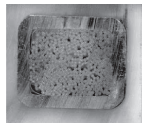
Fig. 1: Picture of the cross section of the conductor sliced at an interval of 10mm.
