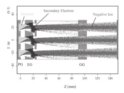
Fig 1. Particle distribution obtained in the simulation.
