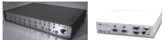
Fig. 3 New FPGA-based timing demodulator (left) and remote power controller (right) boxes: From the 10 th LHD campaign, they have been ready for distribution. They can help us to reduce both the new installation and human maintenance costs for plasma diagnostics.
