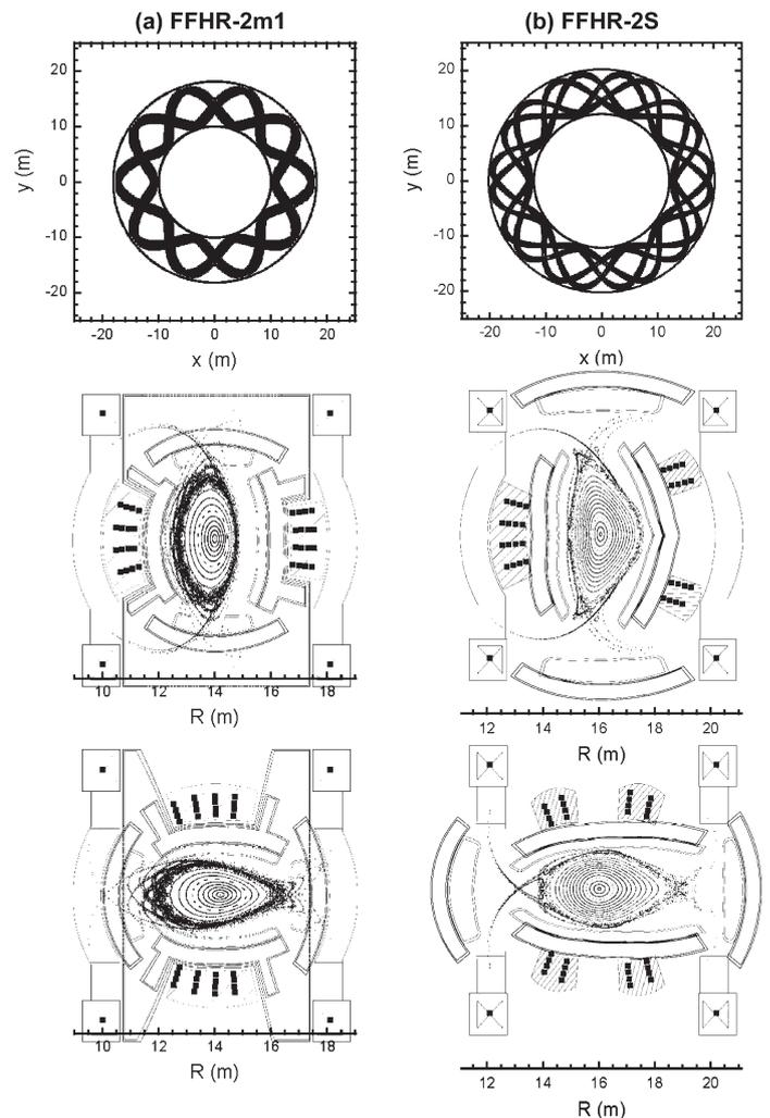
Fig. 1 Plan views of the coils, and magnetic surfaces at two cross-sections for (a) FFHR-2m1 and (b) FFHR-2S.
