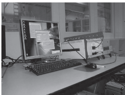
Fig. 21 Test stand for development of the new data acquisition system of the radiation monitoring system
