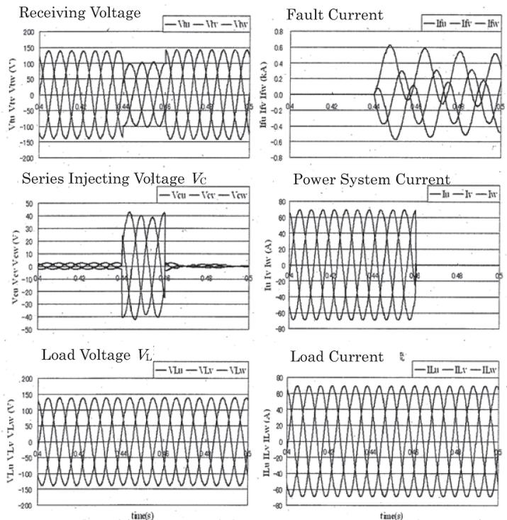
Fig.3. Simulation Result of High Quality B1 Supply System.
