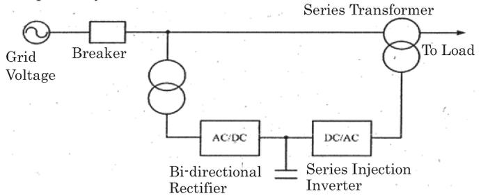
Fig.1. Configuration of the High Quality B1 Supply System.
