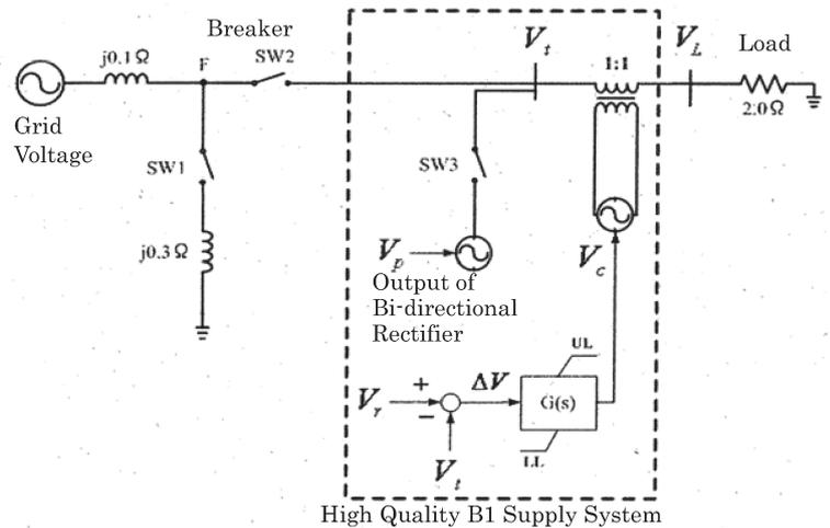
Fig.2. Simulation Model of High Quality B1 Supply System.
