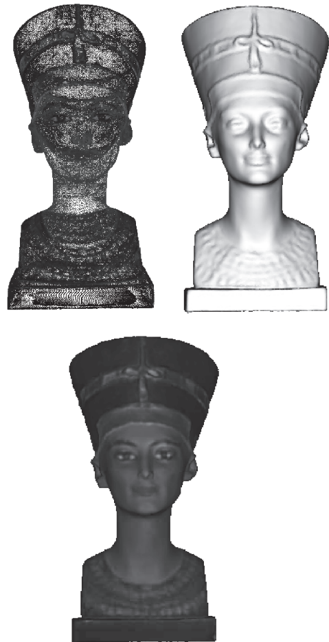
Fig. 1. Example of SLIM surface with colors. Top-left: input point data with colors (860k points), Top-right: SLIM surface model, Bottom: SLIM surface model with local color distribution
