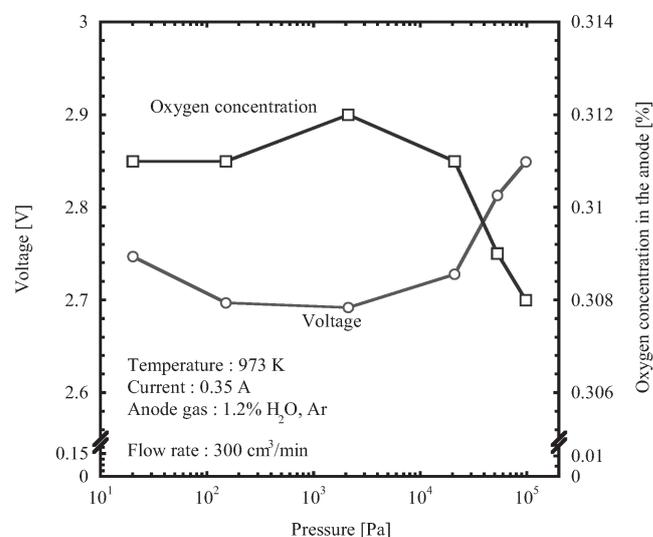
Fig. 1: Pressure dependence of voltage and oxygen concentration in the anode component at 0.35, 973K
