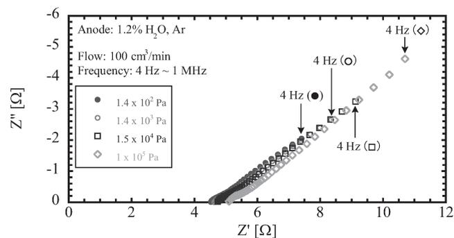
Fig. 2: Pressure dependence of complex impedance measurement in a frequency range of 4 Hz to 1 MHz at 973K
