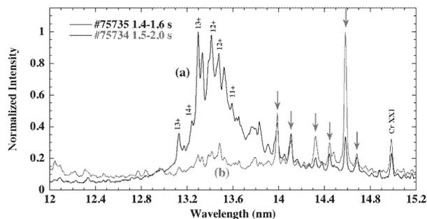
Fig. 2: The two types of EUV spectra (normalized) of tin ions measured in LHD. The case (a) was measured during 1.4–1.6 s in the discharge shown in Fig. 1.
