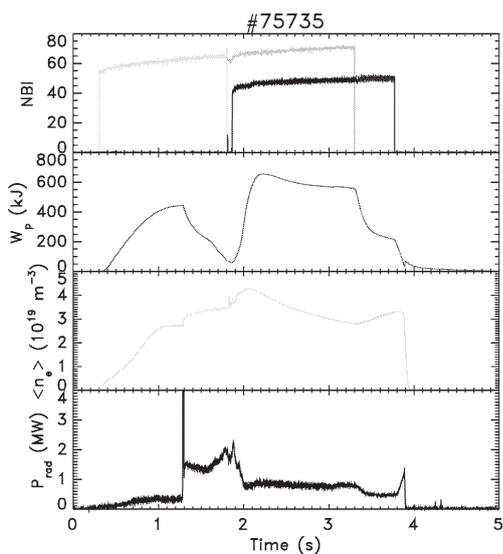
Fig. 1: Time sequences of heating, stored energy ( $W_p$ ) and total radiation power ( $P_{\text{rad}}$ ) in a LHD discharge with a tin pellet injection at 1.3 s.
