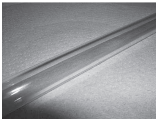
Fig. 2 Photograph of quartz pipe with \text{Er}_2\text{O}_3 thin film.
