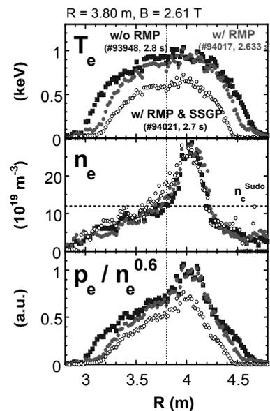
Fig. 2. Radial profiles of (a) the electron temperature, (b) the electron density, and (c) the electron pressure normalized by the gyro-Bohm type density dependence, in the three discharges shown in Fig. 1.
