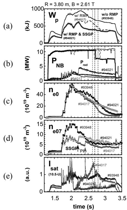
Fig. 1. Typical waveforms in IDB discharges without RMP (#93948), with RMP (#94017), and with both of RMP and SSGP (#94021), where (a) the diamagnetic plasma stored energy, (b) the total heating power, (c) the central electron density, (d) the mantle electron density at  $\rho = 0.7$ , and (e) the ion saturation current measured on a divertor tile are shown from top to bottom.
