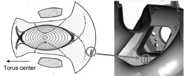
Fig. 1 Position of ion flux monitor on first-wall.
