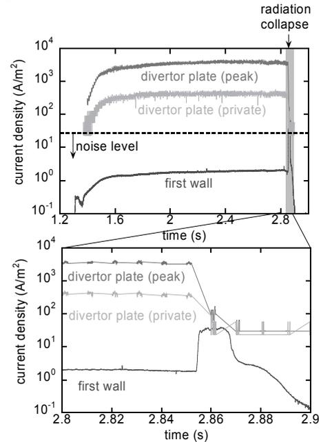
Fig. 2 Typical time evolutions of ion saturation current measured at first-wall and divertor.
