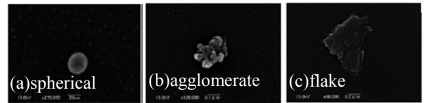
Fig. 2. SEM images of (a) spherical dust, (b) agglomerate, and (c) flake collected in the helicon discharge chamber.
