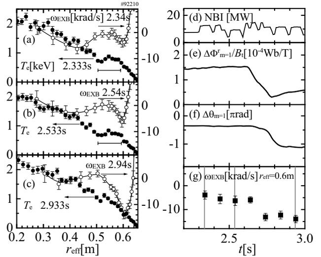
Fig.1 (a-c) Radial profile of  $T_e$  (closed) and  $\omega_{E \times B}$  flow (open). (d-g) Time evolution of NBI,  $\Delta\Phi_{m=1}^r/B_t$ ,  $\Delta\theta_{m=1}$  and  $\omega_{E \times B}$ . The island (local flattening at  $r_{\text{eff}} \sim 0.55\text{m}$ ) transits from growth to healing. The  $|\omega_{E \times B}|$  increases with time prior to the island being healed.
