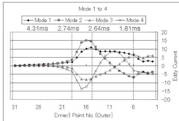
Fig. 3: Low-order (Large time-constant) eddy current distribution in vacuum vessel, which is calculated with EDDY-CAL (JAEA).
