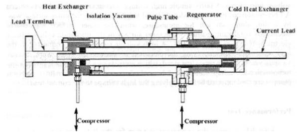
Fig. 1. Schematic diagram of pulse tube current read system<sup>2)</sup>
