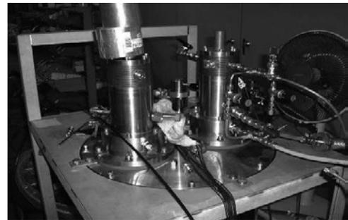
Fig. 2. Photo of pulse tube current lead system (top view)
