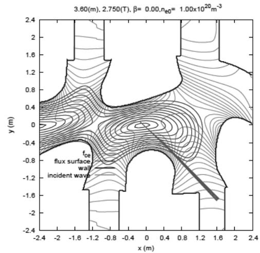
Figure 1: Ray tracing in LHD plasma with density of  $10^{20} \text{ m}^{-3}$  for frequency of 400 GHz.
