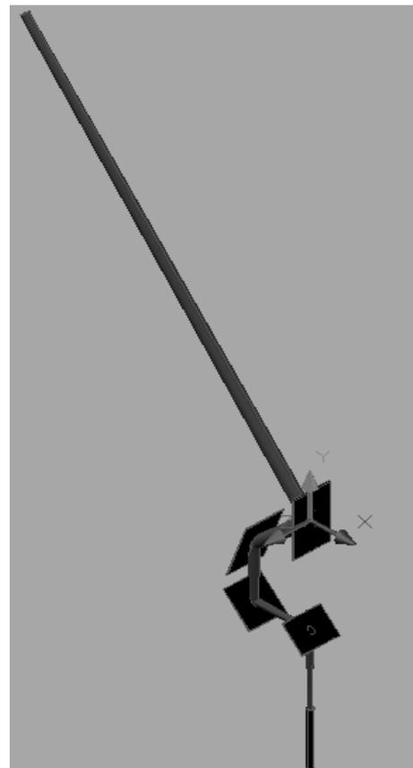
Figure 2: One example of designed transmission system in the LHD vacuum vessel.
