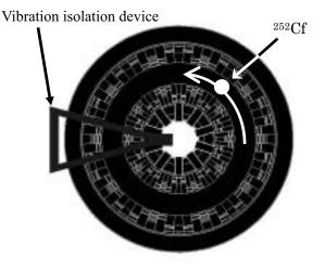
Fig. 1 Simplified geometry of the LHD for neutron transport simulations.
