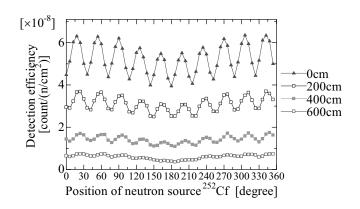
Fig. 2 Detection efficiencies of a fission chamber placed on the center axis and at 0, 200, 400, 600 cm from the equatorial plane of the LHD.
