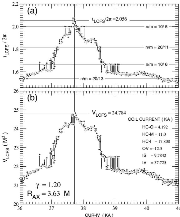
Fig. 2: Change in  $l_{LCFS}/2\pi$  (a) and  $V_{LCFS}$  (b) at IV coil current sweep. Helical coil currents, OV coil current and  $R_{ax}$  are fixed.
