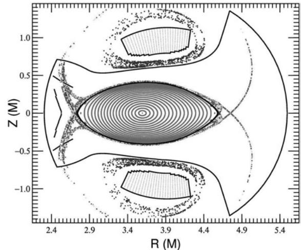
Fig. 4: Poincaré plot of lines of force. Coil currents are shown in Fig.2.
