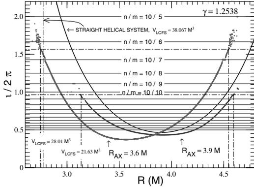
Fig. 1: Effect of inward shift of magnetic axis for the rotational transform  $l/2\pi$ . The positions of the last closed flux surface are plotted together with the values of the plasma volume  $V_{LCFS}$ . Results for the straight helical systems are also shown.
