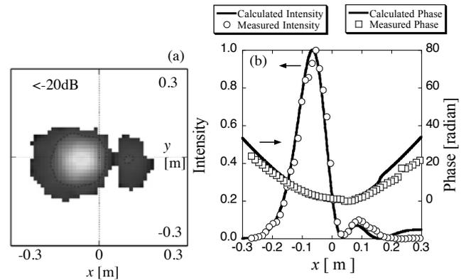
Figs.2 (a): Contour plot of radiated intensity pattern. (b): Calculated and measured intensity and phase profiles in the steering  $x$  direction.
