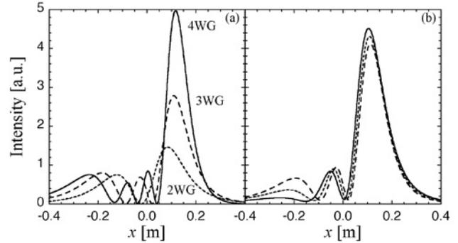
Fig.1: Radiated intensity profile in the steering  $x$  direction at various numbers of 1 dimensional waveguide elements and waveguide sizes.
