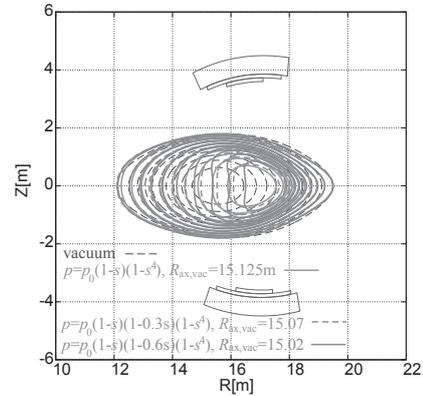
Fig. 2: Equilibrium magnetic surface structure for 3 different pressure profiles ( $s$ : normalized toroidal flux).
