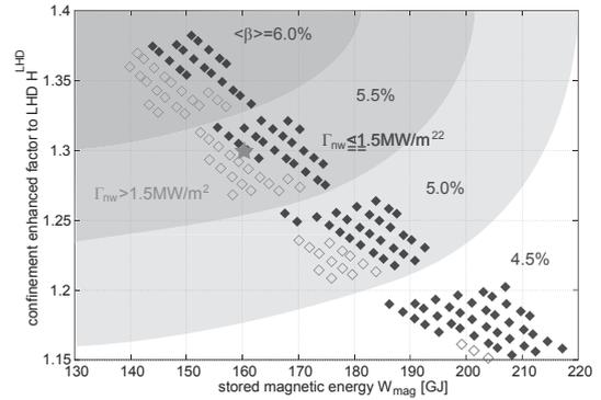
Fig. 1: The stored magnetic energy vs. the required confinement improvement factor for the design points with fusion output  $\sim 3$  GW.
