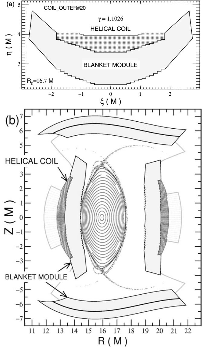
Fig. 2: (a) Cross section of Helical coil and blanket module. (b) Poloidal cross section of magnetic surface, divertor-leg and blanket module. Thin lines show the similarity extension profiles of the LHD vacuum vessel and helical coils.
