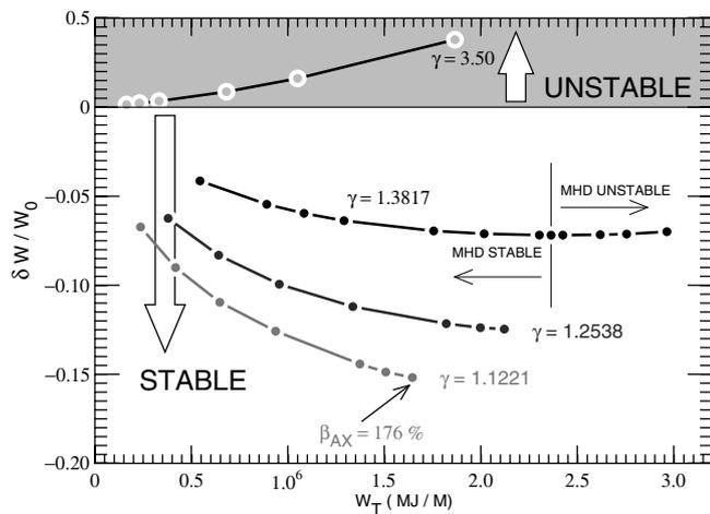
Fig. 1: Variation of MHD potential energy. Abscissa represent the plasma thermal energy stored in the magnetic surface.
