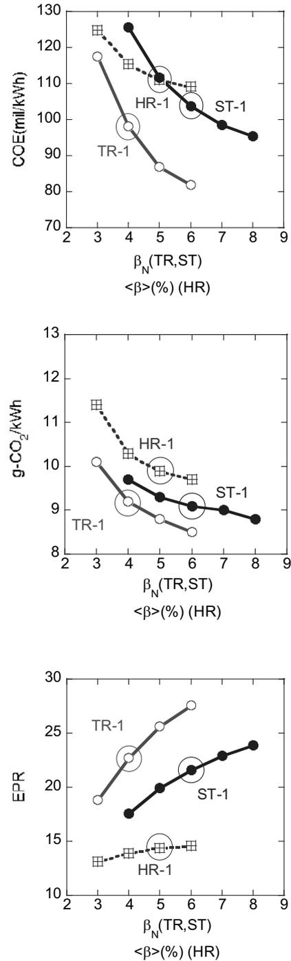
Fig.1 Comparisons on Cost of Electricity (COE) (upper figure), CO<sub>2</sub> emission amounts (middle figure) and Energy Payback Ratio (EPR) (lower figure) for Tokamak reactors(TR), Helical reactors(HR) and Spherical Tokamak (ST) reactors.
