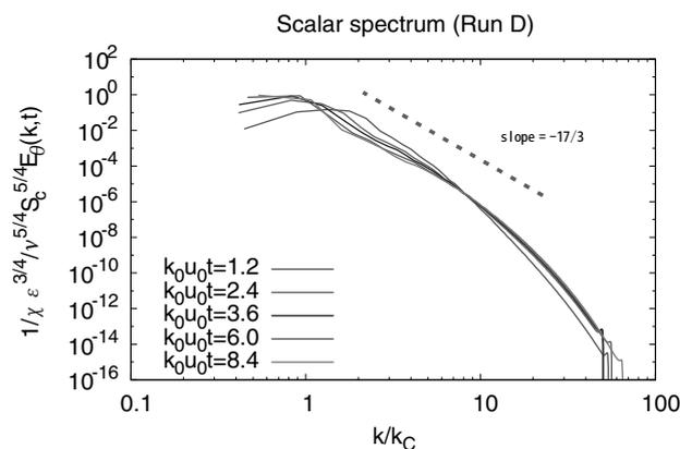
FIG. 1: Evolution of the spectrum of passive scalar variance for  $Sc = 0.01$  for decaying turbulence.
